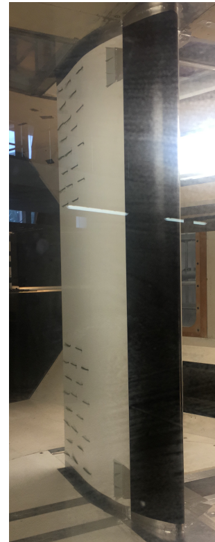
Figure 6. Example of tuft visualisation obtained for a clean airfoil (i.e. no tripping) with a slat at Re = 1.5 \times 10^6 and a small angle of attack.
