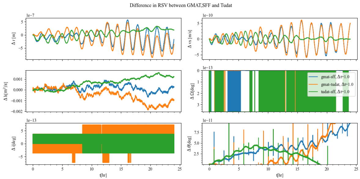
Figure 8.3: Results verification process for the absolute dynamics expressed as the difference between simulation, using the results from GMAT, Satellite Formation Flying (SFF) software, and Tudat. All simulations have been performed for a two-body problem with a fixed 1 second RK4 integrator.
