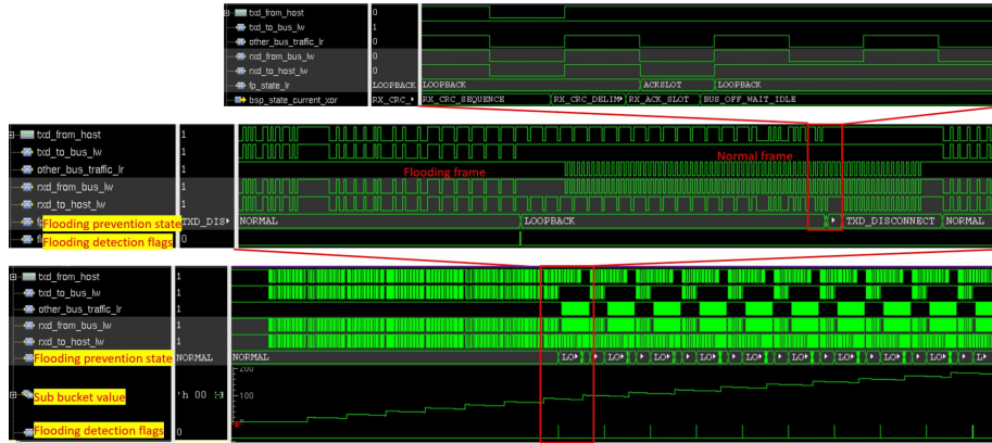
Figure 6.11: Simulation waveform in which the flooding is from other branches via the the gateway
