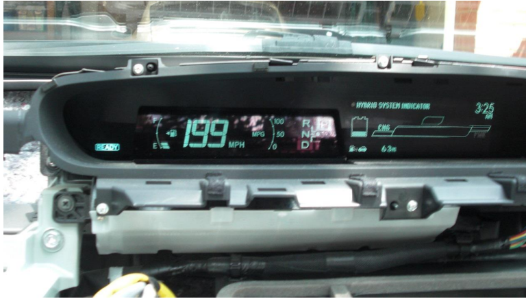
Figure 1.4: The compromised speedometer can be controlled to display any value[19]
