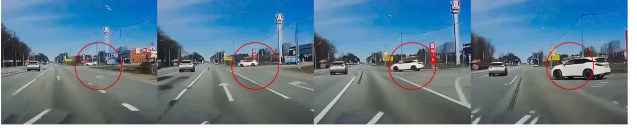
(a) Video stream for a potential collision. The neighbouring vehicle (white) stays at the same bearing (the red circle) and becomes larger when on a crossing course with the subject vehicle (Crashdashes, 2023). Here the bearing is the orientation in the field of view in which another object is observed.
