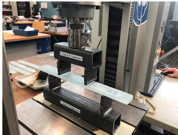
Fig. 15 The four-point bending test for sample 5 to 10, photo by author.
