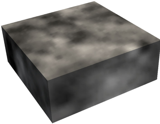
Figure 3. Soil spatial variability for a typical realisation (soil domain 5 \times 5 \times 2 \text{ m} and \theta_{\text{In } c_u} = 2 \text{ m} ).
