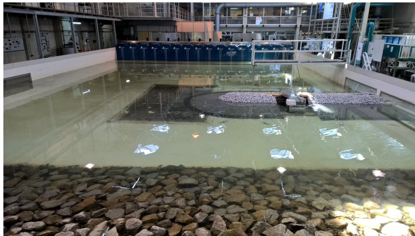
Figure 4.1: Wave basin used for the UPorto tests.
