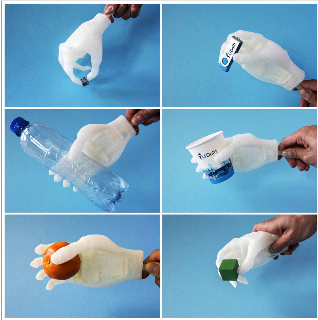
Figure 6. Grasping patterns. Pinch grasping (top left and right), power grasping (middle left and right), spherical grasping (bottom left), and tripod grasping (bottom right).
