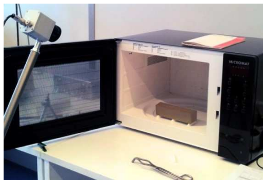
Fig. 2: Test setup with gypsum specimen
