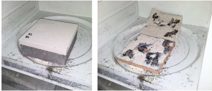
Fig. 4. Specimens with gypsum plaster prior to (top) and after (bottom) microwave treatment
