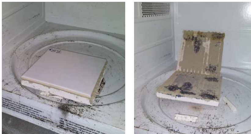
Fig. 5. Specimens with tiles prior to (top) and after (bottom) microwave treatment
