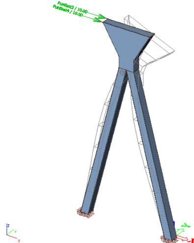
**Figure 2.4** Estimation of the horizontal stiffness of the column using SCIA Engineer
