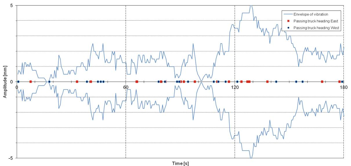
Figure 5.8 Envelope of the vibration's amplitude and the time of passing trucks
