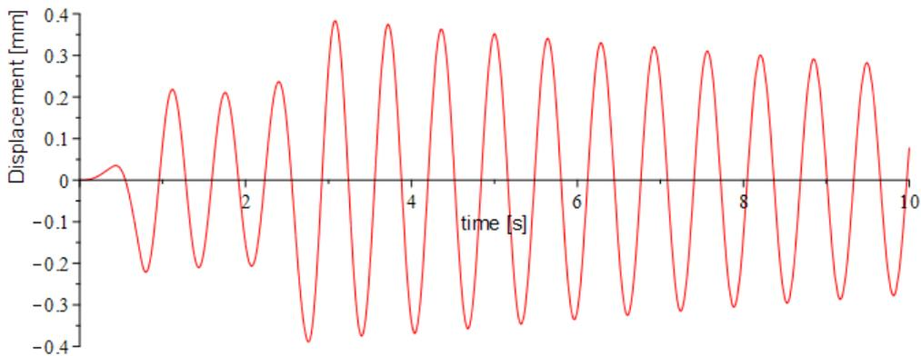
**Figure 4.4** Analytical solution of the structural response of a SDOF to two truck pulses with a time difference of 2 seconds in between the pulses
