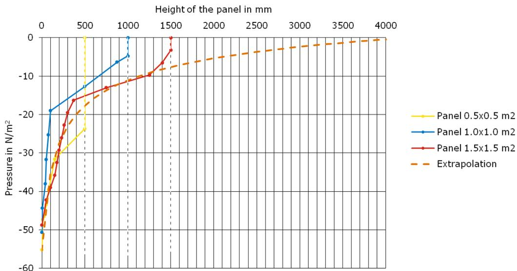
**Figure 3.9** Pressure along the height in the middle of the panels with a surface area of: 0.25; 1.00 and 2.25 m<sup>2</sup>. The pressure along the height of the largest panel is extrapolated this is approximated with equation 3.5.
