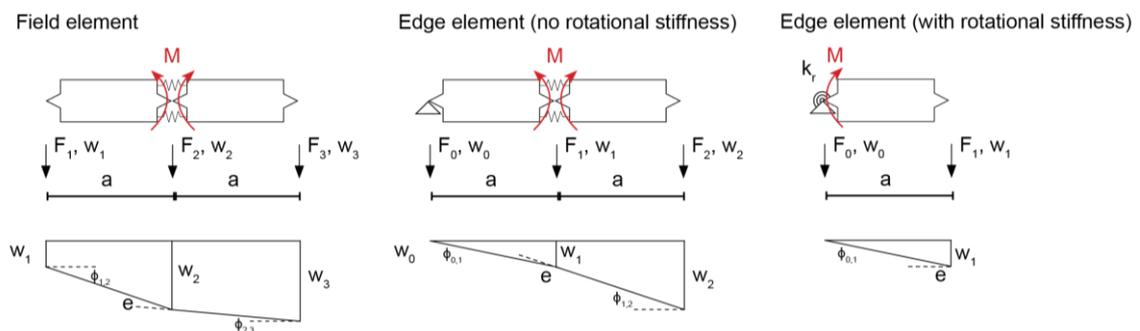
**Figure 4.9** Determination of the stiffness matrices of the field and edge element with and without rotational stiffness
