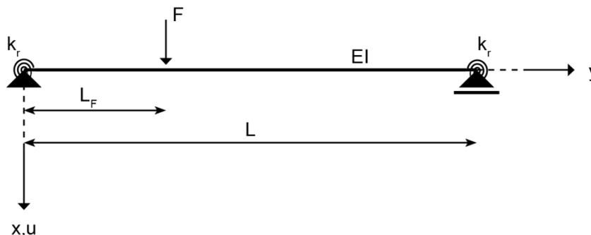
**Figure 2.2** Mechanical scheme for calculation of the horizontal deflection of the beam with rotational springs at the supports. In general the x-axis is parallel to the traffic flow.
