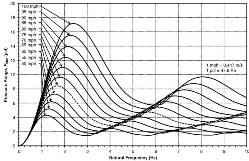
Figure 3.3 Vertical truck-induced design pressure from Hosch & Fouad (2010)
