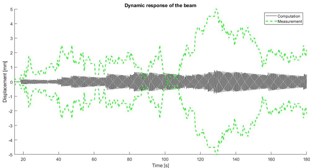
**Figure 5.9** Results of the computation compared to the results from the measurements (beam: simply supported discretized with 53 nodes)
