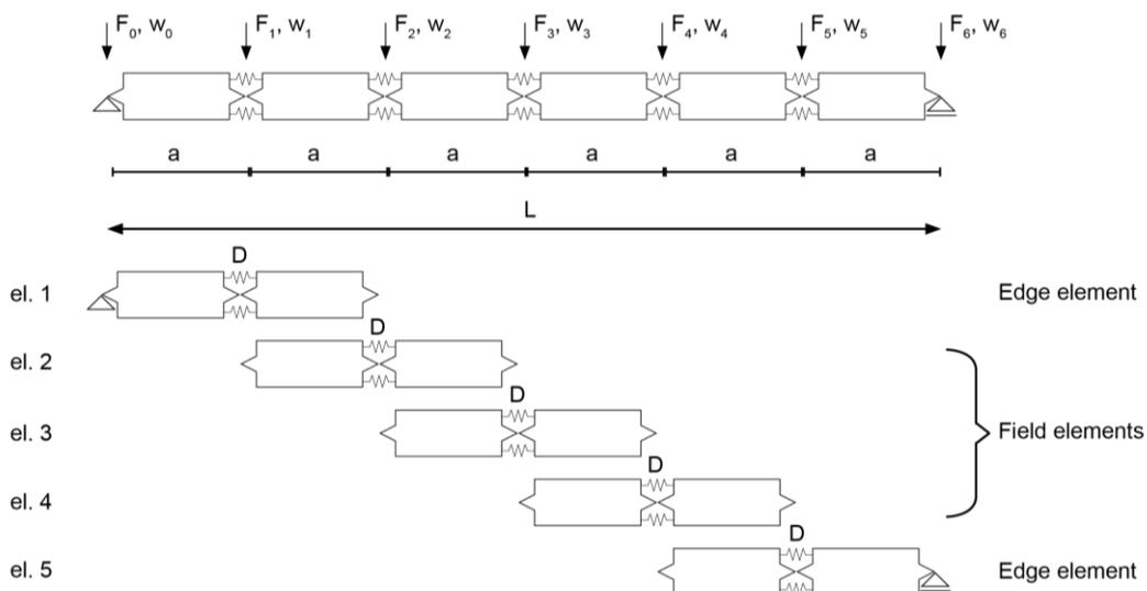
Figure 4.8 Division of the beam into 5 coupled segments, 2 edge elements and 3 field elements
