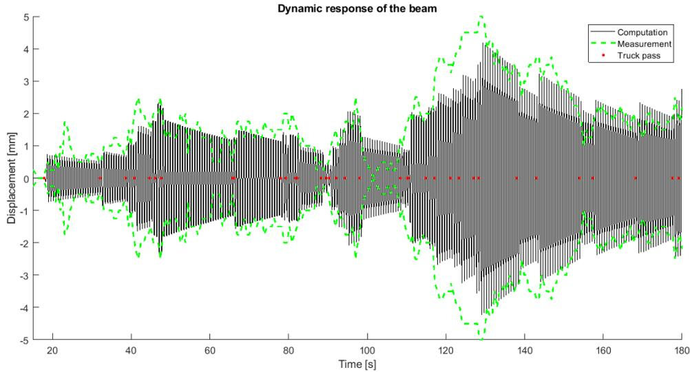
**Figure 5.12** Response of the beam at the specific detail. Specific truck times shifted with  $\pm 0.2$  s and load multiplied with a factor 4.5 to obtain fitted results compared to the measurements (beam: simply supported with rotational springs, mass of the signboards is non-uniformly distributed and the beam is discretized with 27 nodes)
