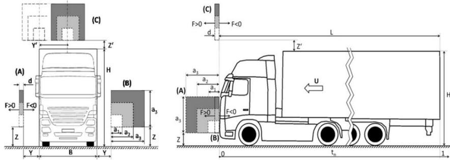
Figure 3.4 Test set-up full scale measurements by Lichtneger & Ruck (2014)
