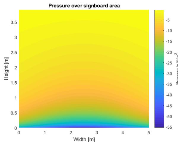
**Figure 3.11** Pressure variation over the area of the signboard for the under pressure peak
