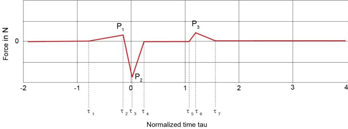
Figure 4.2 Pulse load divided into 7 parts
