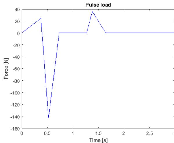
**Figure 3.12** Pulse load on a signboard for a trailer truck based on the extrapolated results of Lichtneger & Ruck (2014). Length of the truck 16.6 m; height of the truck; 4 m; width of the truck 2.6 m; distance between truck and signboard 1.2 m. Signboard 5 m wide and 3.9 m high.
