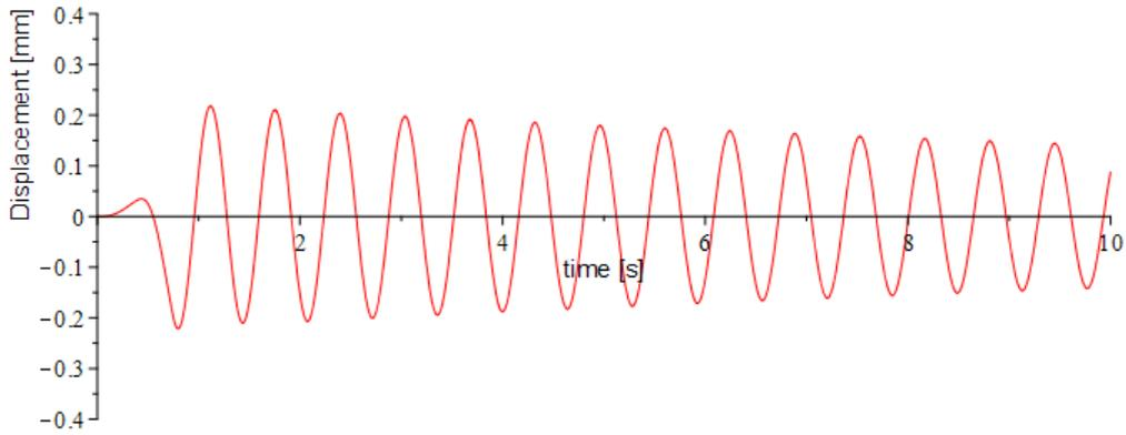
**Figure 4.3** Analytical solution of the structural response of a SDOF to one truck pulse
