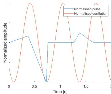
**Figure 4.12** The shape and length of a truck pulse load compared to an oscillation in the natural frequency of the beam (i.e. 1.57 Hz)
