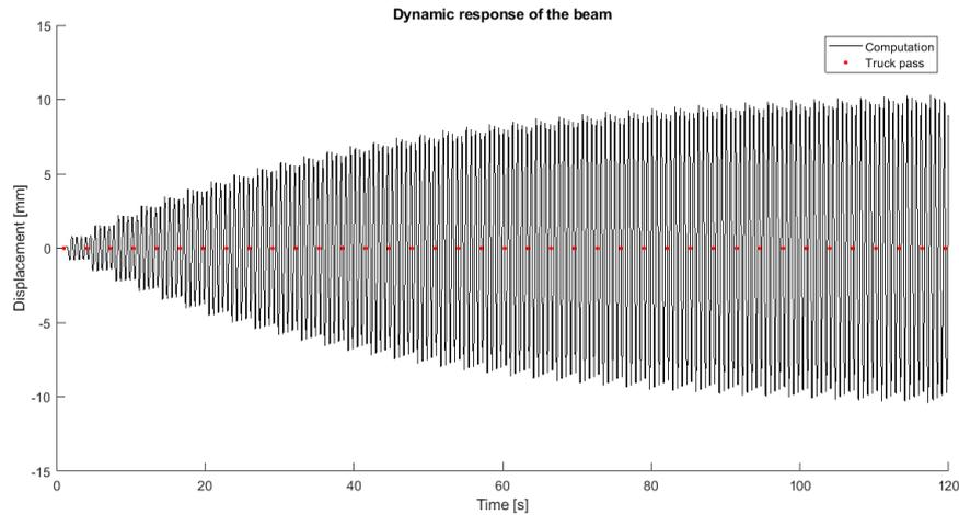
**Figure 6.1** Response of the truss beam at mid span due to 39 trucks at lane 2 in eastward direction with at time distance of 3.12s
