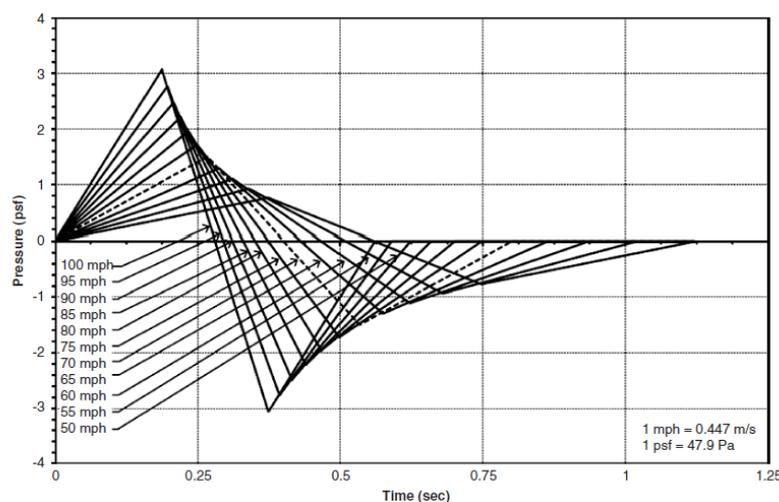
Figure 3.2 Vertical truck-induced wind gust pulse for one truck from Hosch & Fouad (2010)
