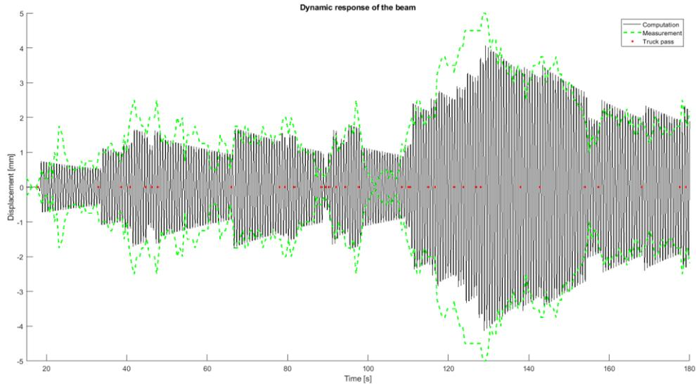
**Figure 5.10** Response of the beam at the specific detail. Specific truck times shifted with 0.20 s and pulse multiplied with a factor 4.2 to obtain fitted results compared to the measurements (beam: simply supported discretized with 27 nodes)
