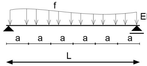
Figure 4.6 Beam divided into 6 segments of length 'a'
