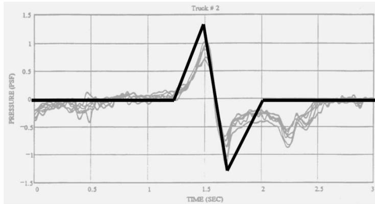
Figure 3.13 Typical truck pulse simplified by Ginal (2003)
