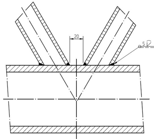
Figure 6.5 Weld detail of the chord-brace connection (2012 series)
