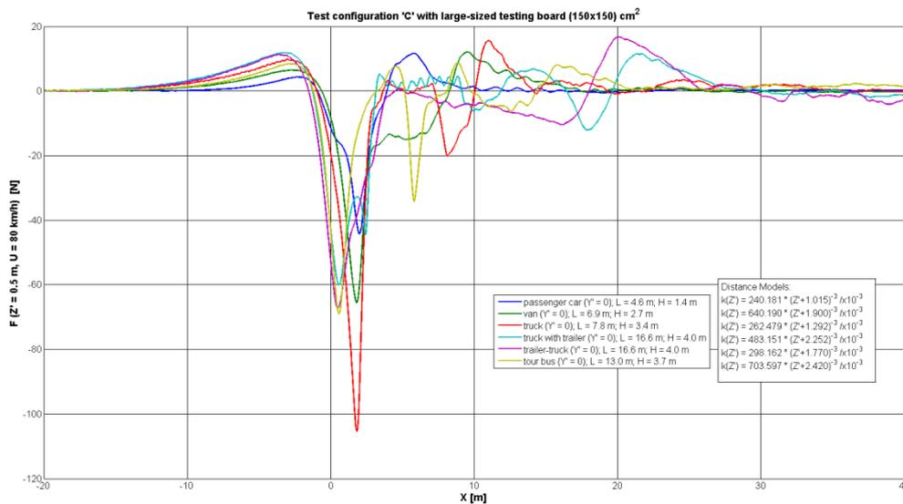
**Figure 3.8** Pulses of vehicle induced wind loads for different type of vehicles on a signboard of  $1.5 \times 1.5 \text{ m}^2$  and  $0.5 \text{ m}$  above the vehicle. Figure from the full scale measurements from Lichtneger & Ruck (2014)
