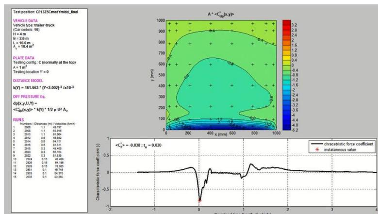
Figure 3.6 Pressure profile in time and pressure distribution on a panel of  $1.0 \times 1.0 \text{ m}^2$ , screenshot of the pressure distribution at the suction peak (Lichtneger & Ruck, 2014)
