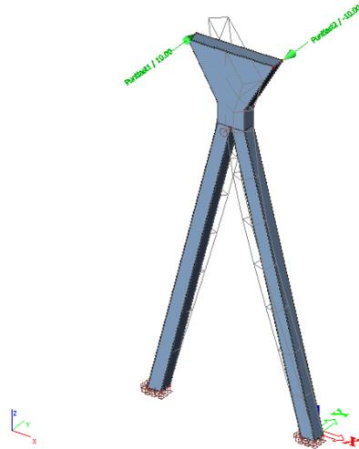
**Figure 2.3** Estimation of the rotational stiffness of the column using SCIA Engineer
