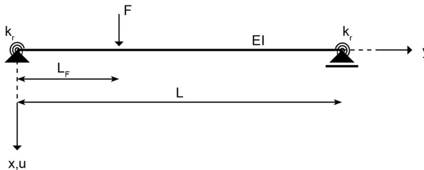
**Figure** Mechanical scheme for calculation of the horizontal deflection of the beam. The principle of superposition is used to calculate the deflection at mid span
