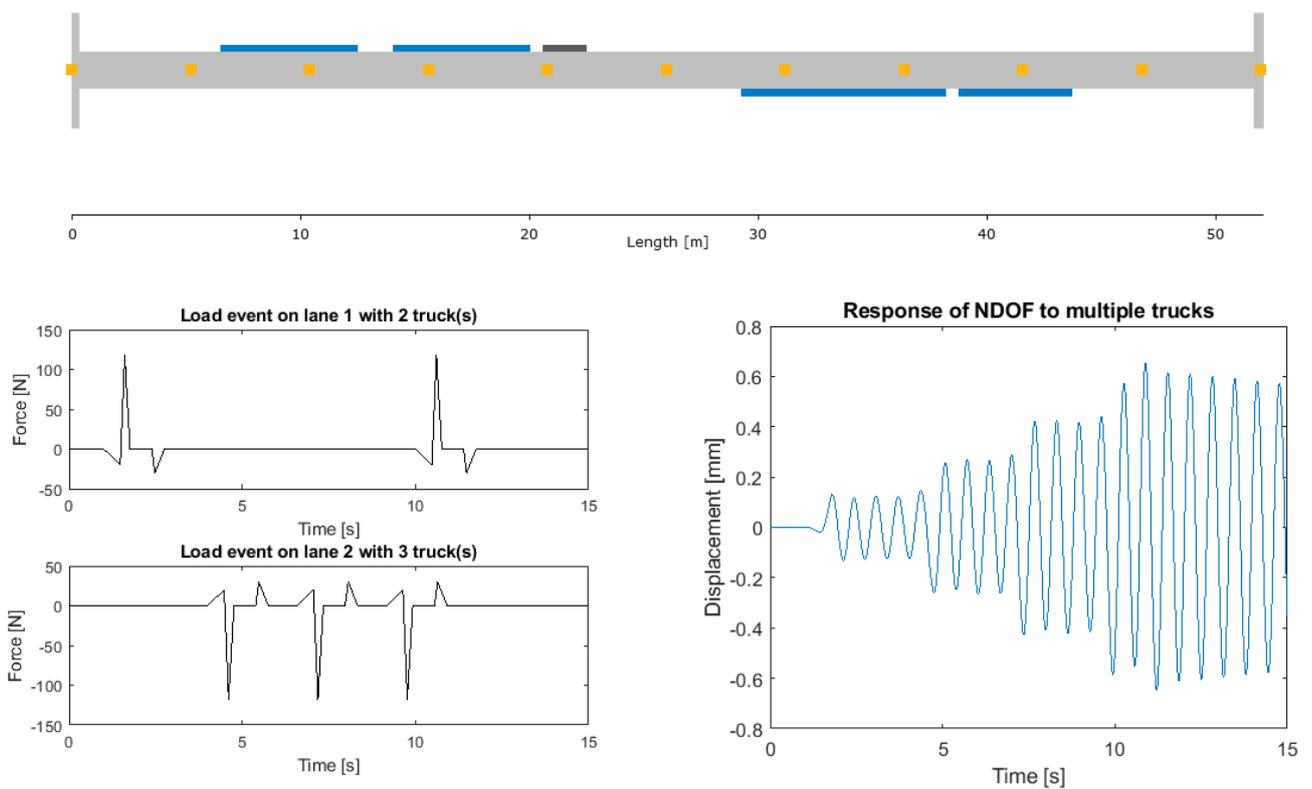
**Figure 4.11** Computation of the structural response to 5 truck pulses at two lanes (node 3 and 8 in the top figure). The displacement of the 6<sup>th</sup> node is shown, this is the node at mid span of the beam.
