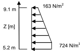
Figure 3.1 Pressure over the height of the signboard
