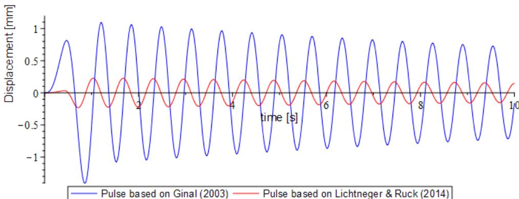
**Figure 4.5** Analytical solution of the structural response of a SDOF to one truck pulse based on Lichtneger & Ruck (2014) and Ginal (2003)
