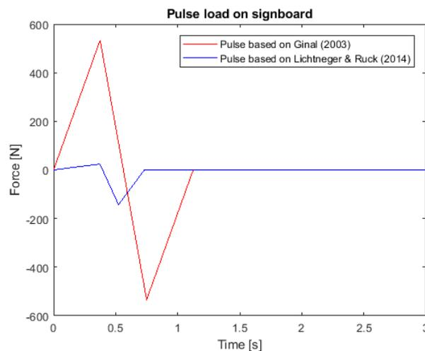
Figure 3.14 Comparison pulses based on data of Lichtneger & Ruck (2014) and results of Ginal (2003)
