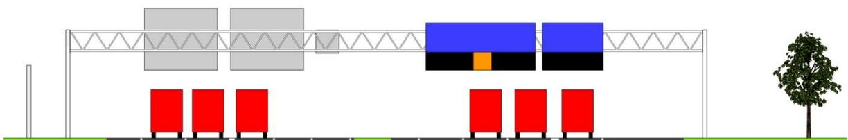
**Figure 5.11** The largest panel size from the measurements of Lichtneger & Ruck (2014) is shown in orange and is compared with the size of the signboards.
