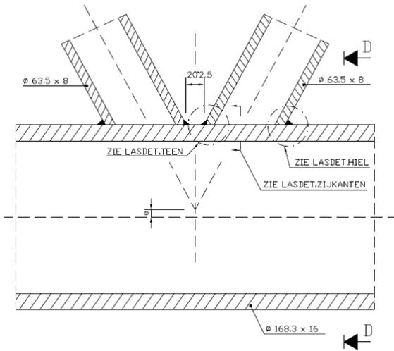
Figure 6.4 Weld detail of the chord-brace connection (2005 series)
