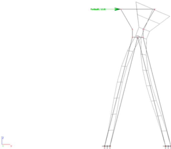
**Figure** Deformed structure due to the second load configuration (bending moment)
