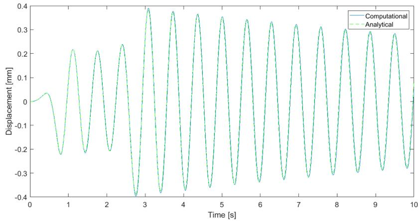
**Figure 4.10** Analytical solution from Maple and computational solution from MATLAB for two truck pulses with time difference of 2s
