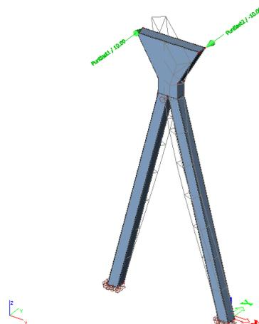
Figure Deformed structure due to the first load configuration (torsion moment)
