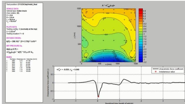
**Figure 3.7** Pressure profile in time and pressure distribution on a panel of  $1.5 \times 1.5 \text{ m}^2$ , screenshot of the pressure distribution at the suction peak (Lichtneger & Ruck, 2014)
