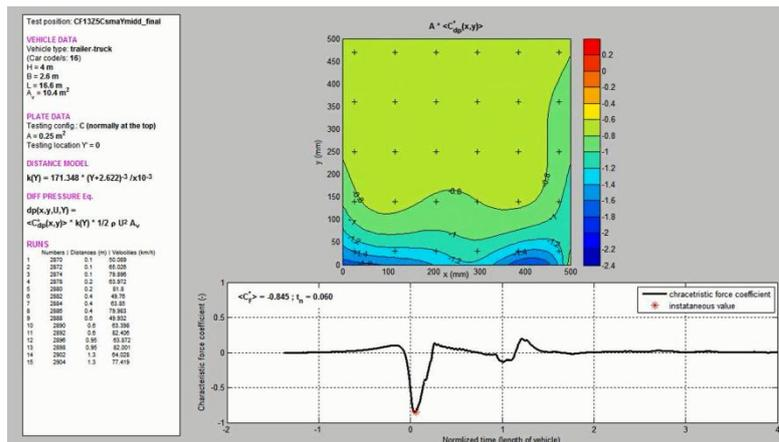
Figure 3.5 Pressure profile in time and pressure distribution on a panel of  $0.5 \times 0.5 \text{ m}^2$ , screenshot of the pressure distribution at the suction peak (Lichtneger & Ruck, 2014)
