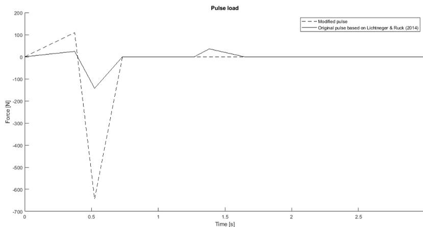
**Figure 5.13** Modified general pulse based on fitting of the computation to the measurements and original pulse based on literature research
