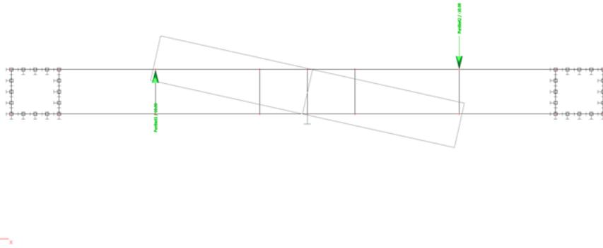
**Figure** Top view of the deformed structure due to the first load configuration (torsion moment)
