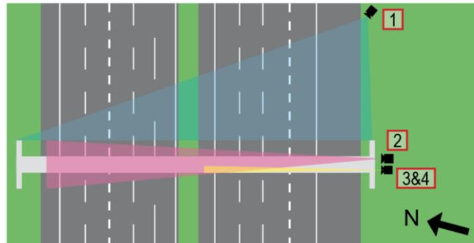
**Figure 5.2** Set-up of the cameras for measurements. The camera with the blue area gives an overview of the situation, the camera with the pink area gives an overview of the vehicle's speed and the cameras with yellow area are focussed on two specific details
