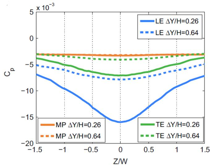
**Figure 3.10** Pressure variations in horizontal direction at two different heights (Mattana et al., 2014). In this figure  $Z$  is the horizontal coordinate,  $W$  is the vehicle width,  $\Delta Y$  is the distance between the vehicle and the object,  $H$  is the vehicle height and  $C_p$  is a pressure coefficient. LE stands for leading edge, MP for mid-point and TE for trailing edge.
