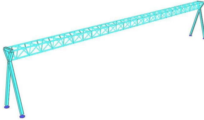
**Figure 6.3** MatrixFrame calculation model with only bar elements connected rigidly. The governing location is the K-joint at mid-span in the upper plane of the truss
