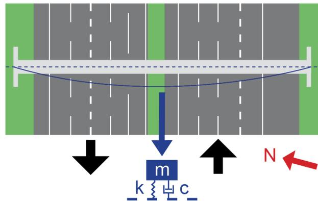
**Figure 4.1** Simplification of the system into a damped mass spring system. Top view of the situation; in white the sign support structure, in grey the carriageways, in green the verge and the first mode shape in blue. The orientation to the north is shown in red
