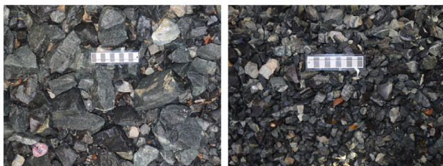
Fig. 10. Photo of surface gravel for the poorly-sorted revetment after standard wave conditions (38 h) at (left) the toe of the revetment and (right) the crest of the revetment. The total length of the scale bar is 198 mm.
