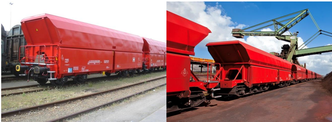
Figure 4.4: On the left a coal wagon of the type Falns 183 , source www.wikipedia.nl , on the right a picture of the iron ore wagon Falrrs 152 , source EMO dry-bulk terminal
