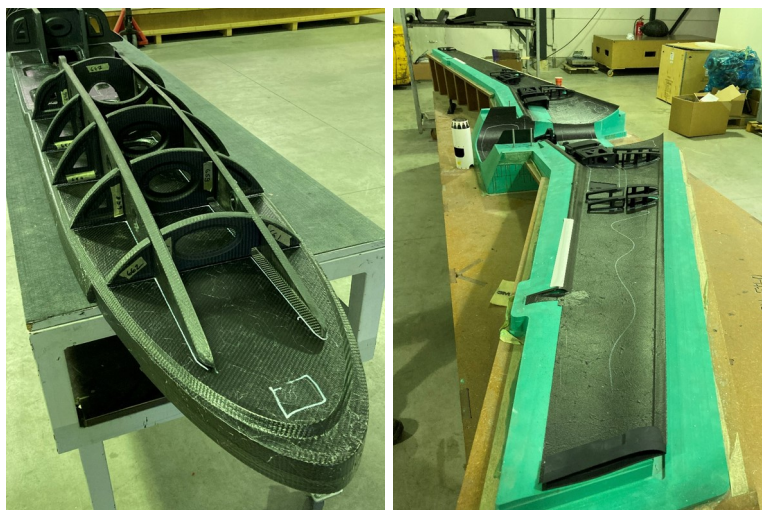
Figure 13. The freshly manufactured fuselage and wings of the DEP-SFD2.
