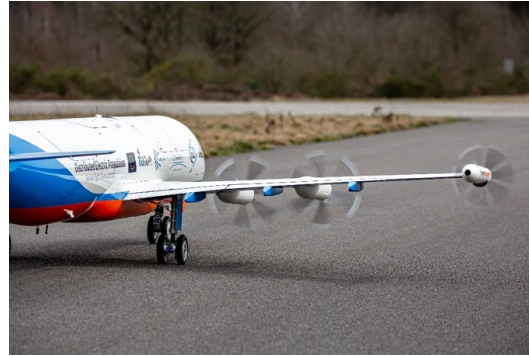
Figure 10. The DEP-SFD during its high speed taxi tests at Deelen Airport.
