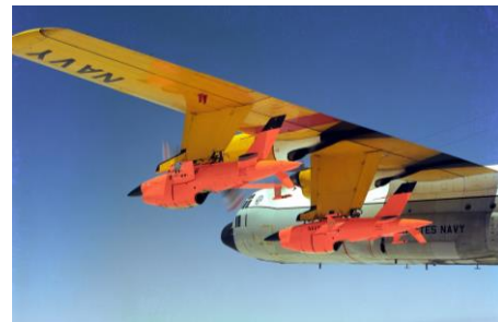
Fig. 4 Firebee target drones mounted under wing of Lockheed DC-130 [8].
