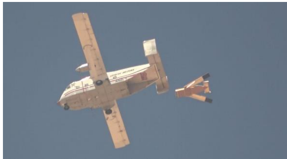
Fig. 3 Deployment flight test of foldable glider [7].
