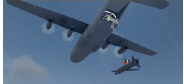
Fig. 2 Airborne recovery of Gremlin (adapted from [5]).
