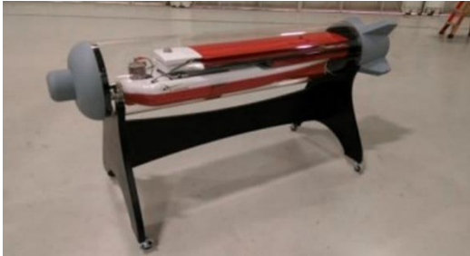
Fig. 1 Dash X UAV in folded configuration [2].
