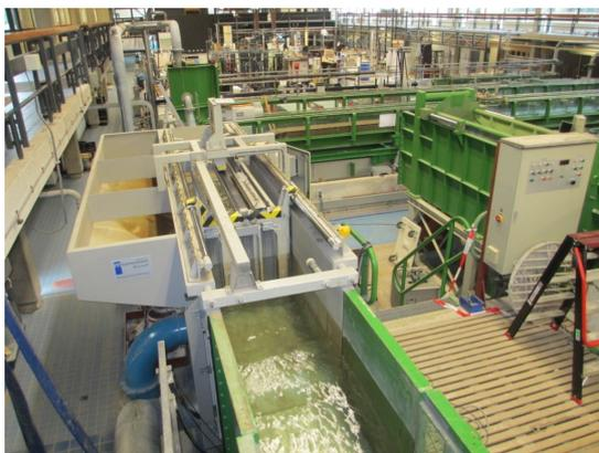
**Figure 3.4:** The piston type wave generator at the start of the flume which generates the waves in these experiments by moving back and forth.
