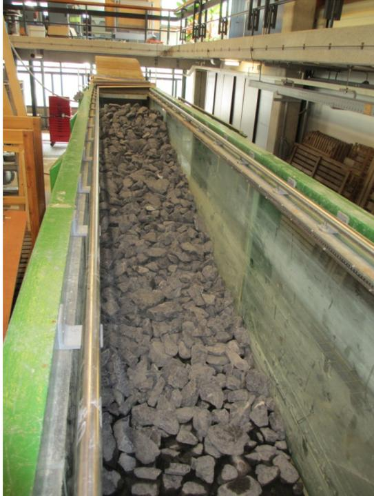
**Figure 3.2:** Photo of rock slope which is used for wave dissipation at the end of the flume.
