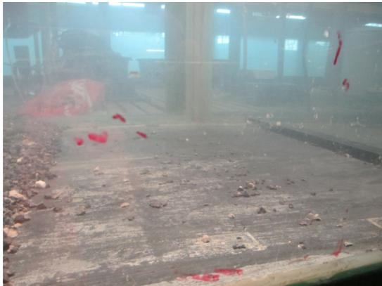
**Figure 4.7:** Photo of stones removed from the profile of the near-bed structure which travel downstream.
