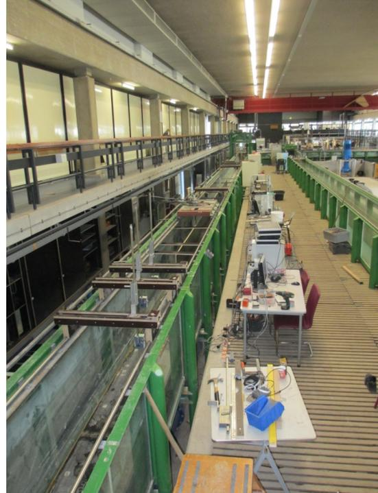
**Figure 3.3:** Wave flume located in the water laboratory of the TU Delft. In the middle the separation board can be seen.
