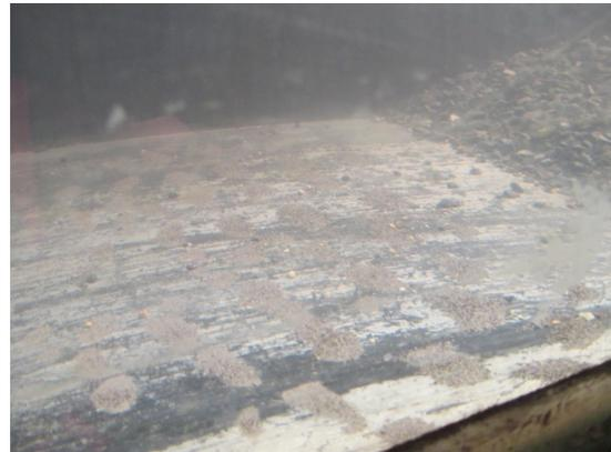
**Figure 4.8:** Photo of accumulating dust and small stones in front of the near-bed structure.
