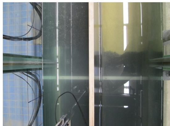
**Figure 3.5:** Overview of the near-bed structures. At both sides of the flume a different near-bed structure can be seen with the separation board in between.
