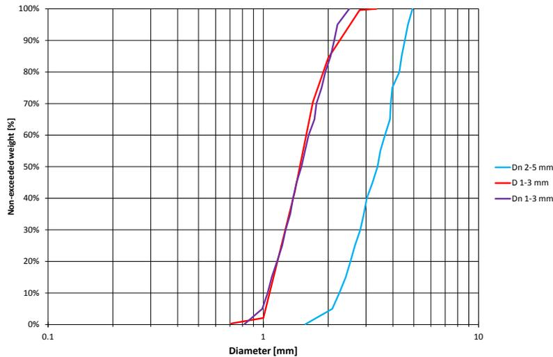
Figure 3.6: Non-exceeded curve for the used test materials.
