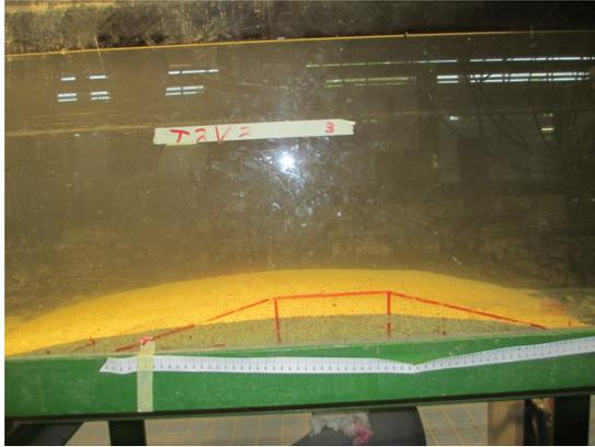
**Figure 4.5:** Photo of test 2Av2 after 10,000 waves where the Gaussian shaped profile can be seen.
