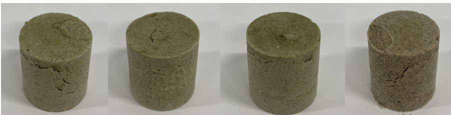
Figure 51: Deficiencies of oven samples
