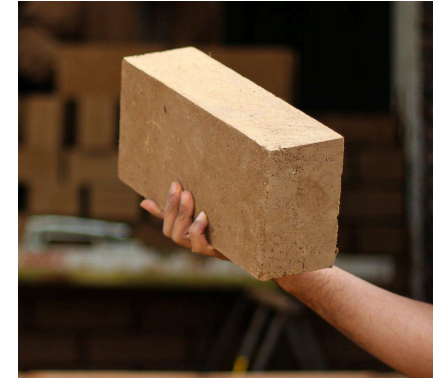
Figure 16: Cow dung stabilised earthen bricks (The Green Village, 2023)
