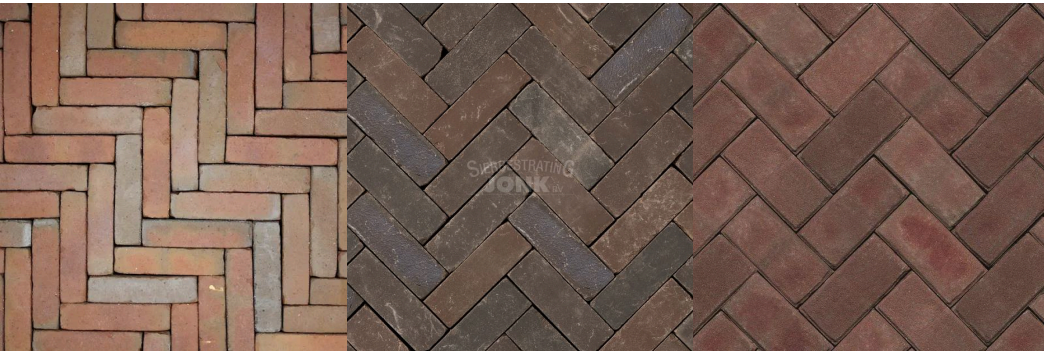
Figure 95: Standard sizes of brick pavers. Waalformaat measuring 200 by 50 by 60 mm (left) (Klinkervisie B.V., n.d.), Dikformaat measuring 200 by 65 by 60 mm (middle) (Jonk Sierbestrating, n.d.), Keiformaat measuring 200 by 100 by 70 mm (right) (Bricks and Stones, 2025).
