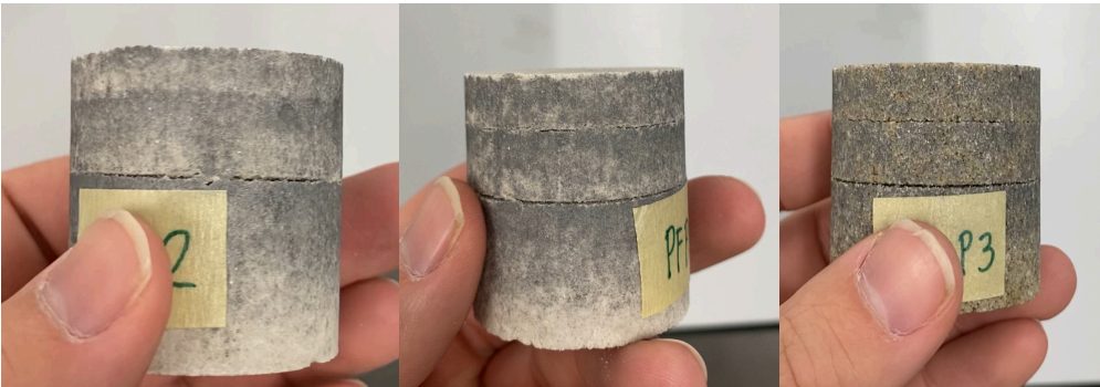
Figure 54: Samples with cracks due to hydraulic press protocol
