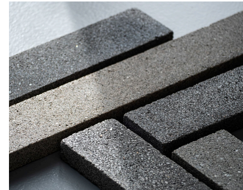
Figure 17: Tiles made with bio-cement (FRONT® Materials, 2024)
