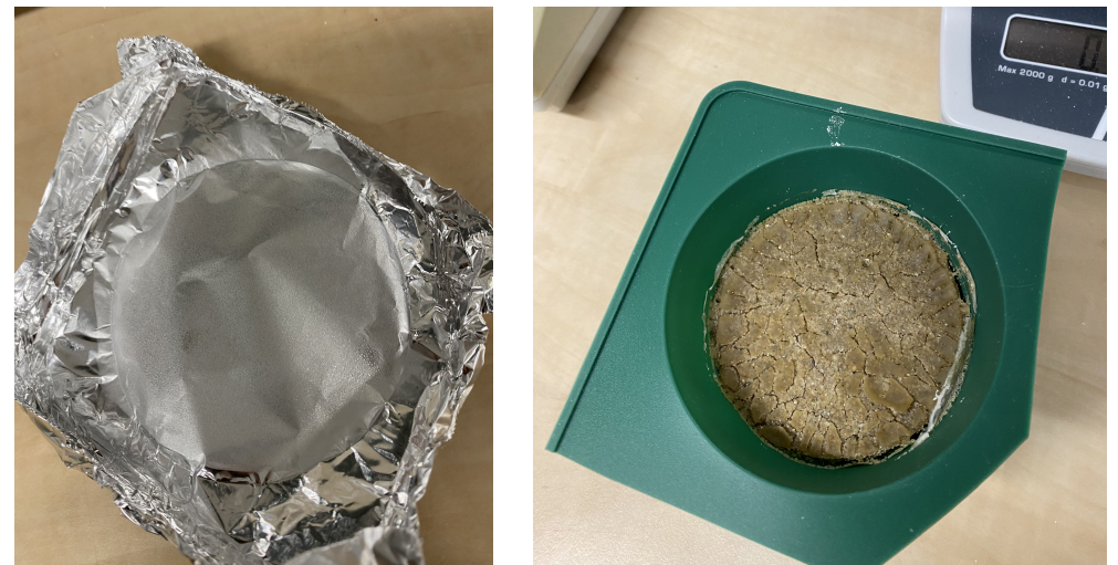
Figure 38: Aluminium foil lid on a silicon mould used for gelatinisation in the oven
