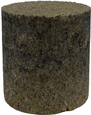
Figure 78: CoRncrete containing 0.250 - 0.500 mm sand grains
