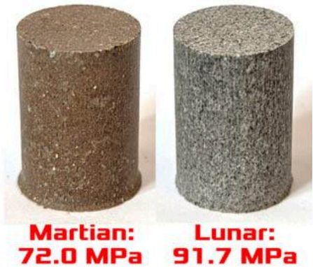
Figure 20: StarCrete manufactured by Roberts & Scrutton (2023)
