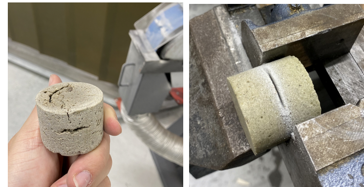
Figure 45: Post-processing CoRncrete with the belt sander (left) and hacksaw (right)
