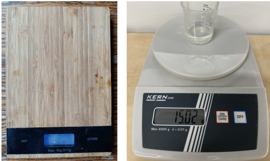
Figure 25: A kitchen scales (left) and Kern EMB 2000-2 scales (right)
