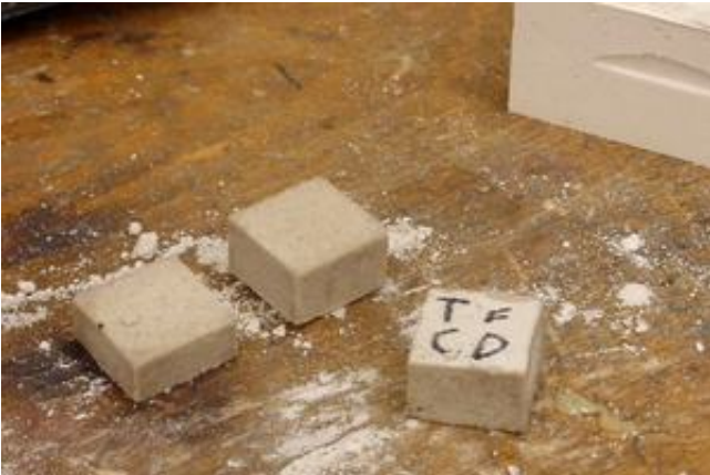
Figure 19: CoRncrete manufactured in the microwave (InstrucTables, 2017)
