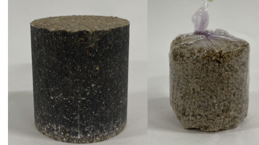
Figure 52: PCC1 made with too much pressure (left) and PCC2 made with too little pressure (right)
