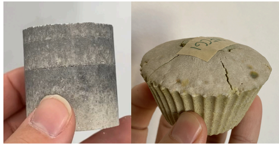
Figure 42: Sample containing Fine sand without pigmentation (left) and with pigmentation (right)
