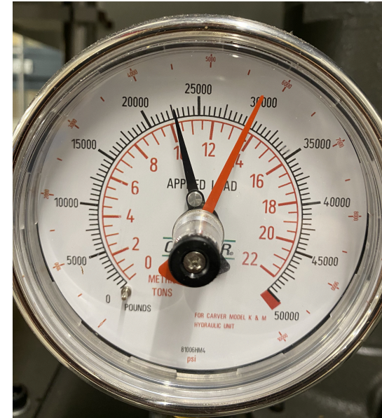
Figure 41: Hydraulic press pressure gauge
