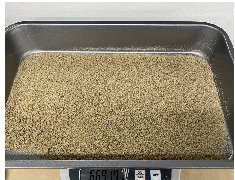
Figure 40: Crushed, dehydrated gelatinised mixture
