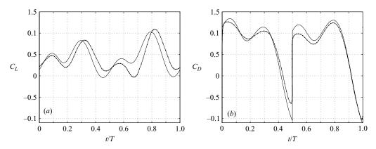
FIGURE 4. Comparison of force coefficients obtained in the present simulations (—) with Wang *et al.* (2004) ( $\bullet$ ). Harmonic wing kinematics with A = 2.8, Re = 75.
