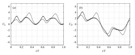
FIGURE 21. Influence of the deviation compared to the harmonic model:  $\bullet$ , harmonic  $\phi$ ,  $\alpha$ ,  $\theta$ ;  $\times$ , harmonic  $\alpha$ ,  $\alpha$  and fruit fly  $\theta$ .
