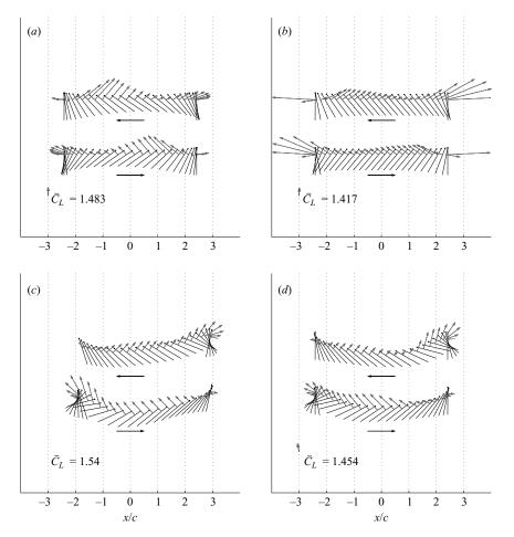
FIGURE 10. Force vectors during each half-stroke. (a) harmonic model, (b) Robofly model, (c) realistic fruit fly model, (d) symmetric fruit fly model.
