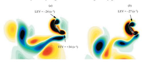
FIGURE 22. Vorticity contours at t = 0.1T (blue: clockwise, corresponding to negative vorticity values): (a) harmonic model, (b) harmonic model with deviation.
