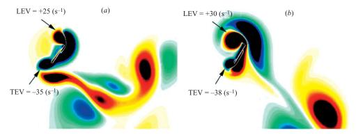
FIGURE 16. Vorticity contours at t = 0.6T (blue: clockwise, corresponding to negative vorticity values): (a) harmonic model, (b) harmonic model with trapezoidal  $\alpha$ .
