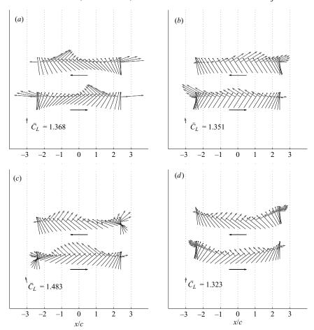
FIGURE 12. Force vectors during each half-stroke. (a) harmonic model with sawtooth  $\phi$ , (b) harmonic model with trapezoidal  $\alpha$ , (c) harmonic model with extra bump  $\alpha$ , (d) harmonic model with deviation  $\theta$ .
