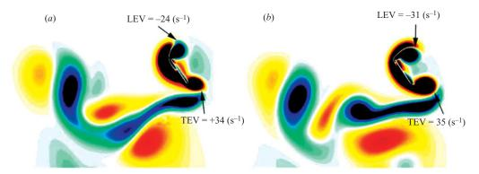
FIGURE 14. Vorticity contours at t = 0.1T (blue: clockwise, corresponding to negative vorticity values): (a) harmonim model, (b) harmonic model with sawtooth displacement.
