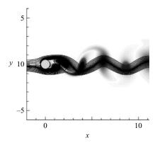
FIGURE 24. General unsteady flow around a fixed cylinder, Re = 150. Vorticity contours are used to visualize the development of a von Kármán vortex street. Streamlines accentuate the wavy pattern in the vortex street.
