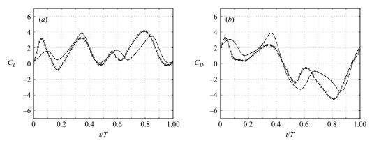
FIGURE 18. Influence of the extra bump in angle of attack:  $\bullet$ , harmonic  $\phi$ ,  $\alpha$ ,  $\theta$ ;  $\times$ , harmonic  $\alpha$ ,  $\phi$  and fruit fly  $\alpha$ .
