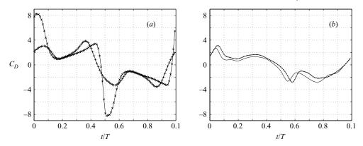
Figure 9. Drag force histories of the baseline kinematic models; +, harmonic model; ×, Robofly model; •, realistic fruit fly model; -, simplified fruit fly model.
