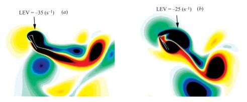
FIGURE 17. Vorticity contours at t = 0.4T (blue: clockwise, corresponding to negative vorticity values): (a) harmonic model, (b) harmonic model with trapezoidal  $\alpha$ .
