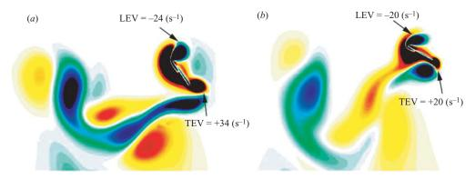
FIGURE 11. Vorticity contours at t = 0.1T (blue: clockwise, corresponding to negative vorticity values) (a) harmonic model, (b) realistic fruit fly model. LEV denotes leading-edge vortex and TEV trailing-edge vortex.
