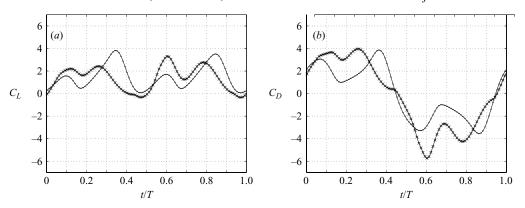
FIGURE 15. Influence of the trapezoidal angle of attack compared to harmonic model:  $\bullet$ , harmonic  $\phi$ ,  $\alpha$ ,  $\theta$ ;  $\times$ , harmonic  $\alpha$ ,  $\phi$  and Robofly  $\alpha$ .
