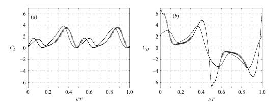
FIGURE 13. Force histories to investigate the influence of the sawtooth displacement compared to the harmonic model:  $\bullet$ , harmonic  $\phi$ ,  $\alpha$ ,  $\theta$ ;  $\times$ , harmonic  $\alpha$ ,  $\theta$  and Robofly  $\phi$ .
