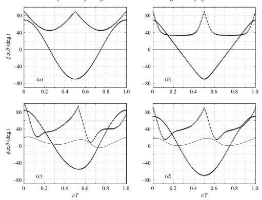
FIGURE 7. Kinematic angles of the different kinematic models. (a) Harmonic model, (b) Robofly model, (c) fruit fly model, (d) simplified fruit fly model. +, displacement;  $\times$ , angle of attack; -, deviation.
