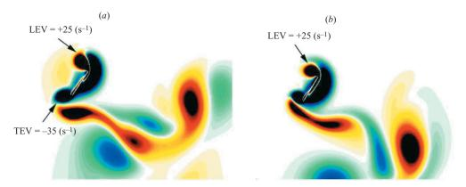
FIGURE 23. Vorticity contours at t = 0.6T (blue: clockwise, corresponding to negative vorticity values): (a) harmonic model, (b) harmonic model with deviation.
