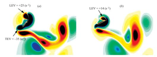
FIGURE 20. Vorticity contours at t = 0.6T (blue: clockwise, corresponding to negative vorticity values): (a) harmonic model, (b) harmonic model with extra bump in  $\alpha$ .
