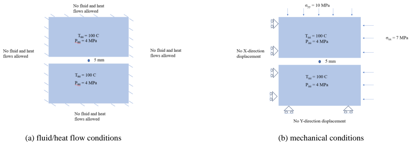
Figure 2: Synthetic model and its boundary and initial conditions
