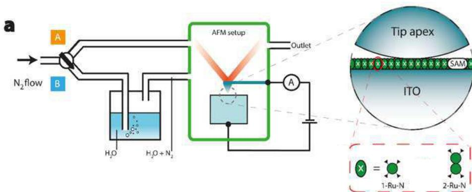
Figure 7.1: Schematic representation of the experimental setup and molecular systems studied.
