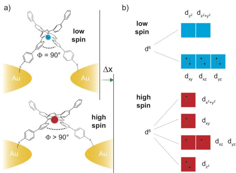
Figure 6.1: Two-terminal mechanically controlled single-molecule junction. a) Sketch of the Fe<sup>II</sup>-based SCO molecular junction and the LS and HS switch triggered by separating the electrodes by  $\Delta x$ . b) Iron II 3d levels involved in the spin-crossover phenomenon.
