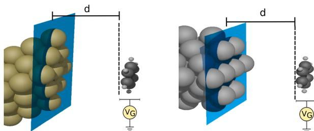
Figure 4.2: Cases studied with a benzene molecule parallel to a gold 111 (left) and a lithium 100 plane (right) lead surface. We show how we define the distance  $d$  and the gate applied over the molecule.
