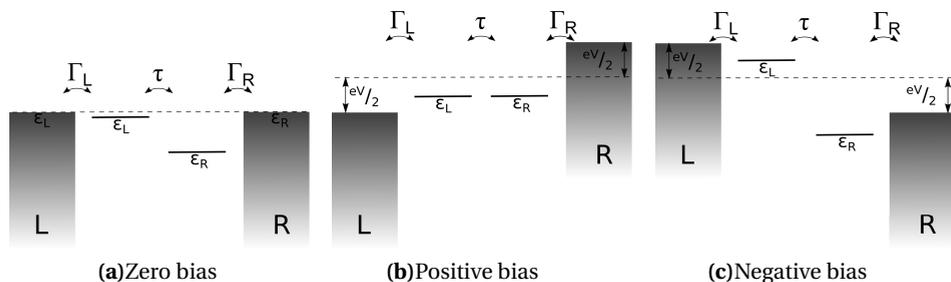
Figure 2.6: Illustration of the charge transport for an asymmetric two-site system. **(a)**, Zero-bias case depicting two molecular levels. **(b)**, With a positive forward bias. The two molecular levels are in resonance and the current is high. **(c)**, With a negative forward bias. The levels are apart from each other, the transport is blocked and the current is low.
