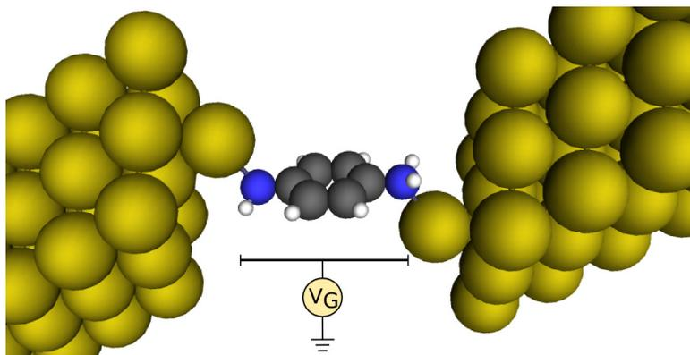
Figure 4.8: Scheme showing the Au-BDA-Au junction and the Gate applied on the molecule.
