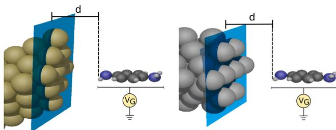
Figure 4.3: Scheme showing the 1,4 BDA and the lead. We show how we define the distance  $d$  and the Gate applied on the molecule for every lead. Gold lead (left), lithium lead (right).
