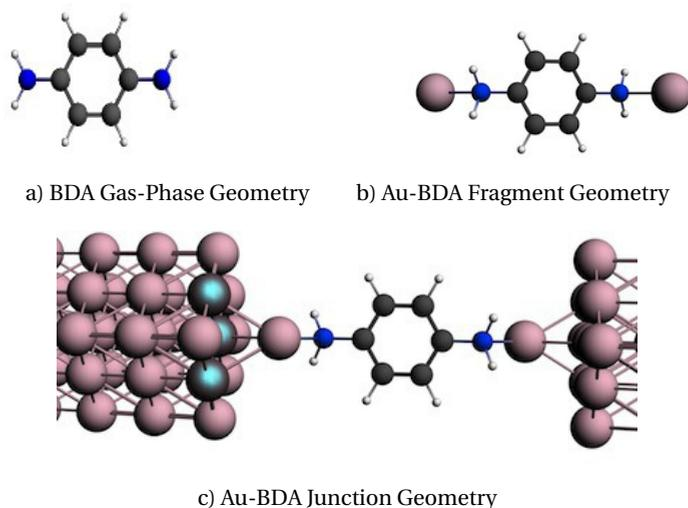
Figure 3.2: Geometries of BDA in (a) gas phase and (b) as a fragment. (c) (1,1) junction geometry. Metal ions are pink-grey, the blue-gray atoms are the substrate atoms coupled to the protruding gold atom. Left and right Au atoms show placement relative to a (111) surface.
