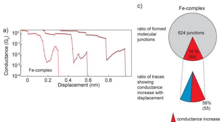
Figure 6.2: a) Conductance measurements of three examples of conductance traces as a function of electrode displacement measured respectively in the presence of the FeII-complex. b) Junction-formation statistics and percentage of molecular junctions showing a conductance increase.
