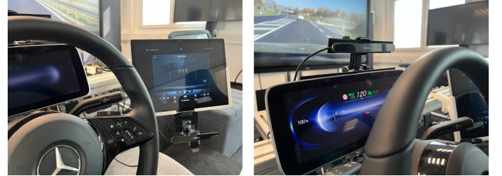
(b) Placement of the Tobii Pro Nano eye tracker below the head unit (left) and above the instrument cluster (right).
