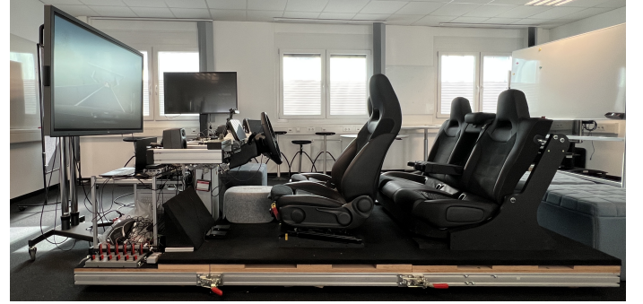
(a) Seating buck with external display placed in front of the dashboard consisting of the steering control, head unit and instrument cluster.
