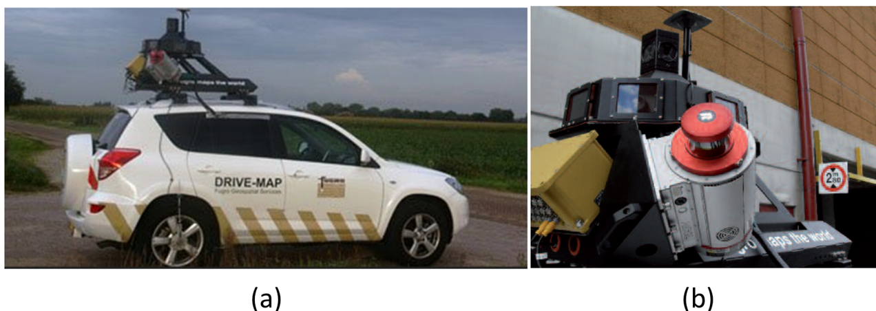
Fig 2. Fugro Drive-map system used for the data acquisition (a) and its LiDAR System (b) (source: Fugro).
