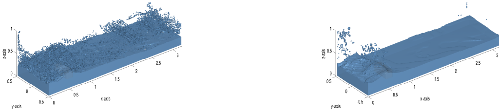
Figure 6: Snapshots at the end of dambreak flow simulations with different algorithms for the displacement of the free surface: original VOF (left) and VOF combined with a local height function (right).
