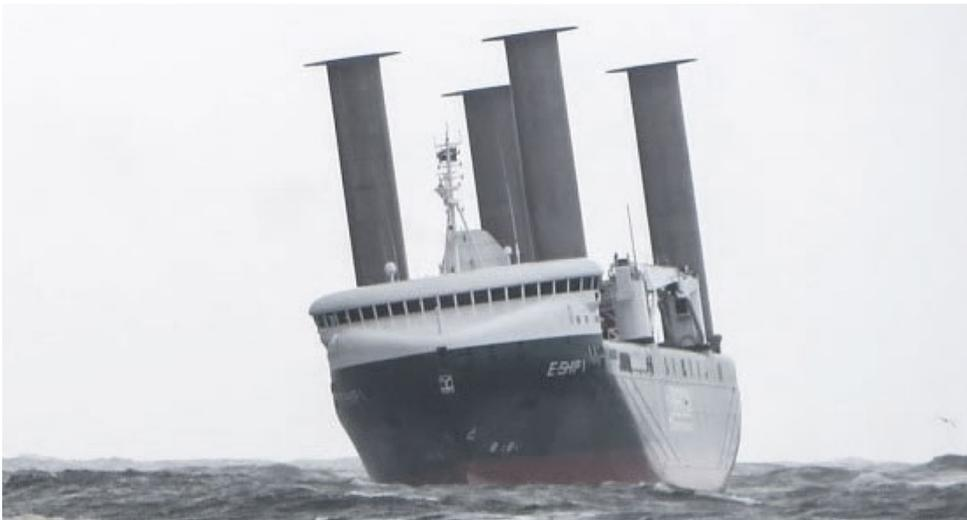
Figure 6.1.: E-Ship1, a 10500 DWT RoLo equipped with four 27 m Flettner rotors. In operation since 2010. (source: [www.enercon.de](http://www.enercon.de)).
