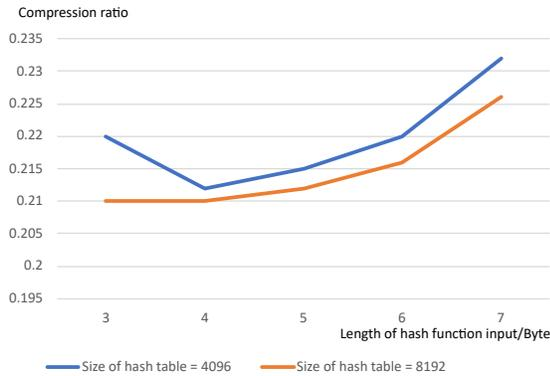
Fig. 4. Compression ratio when using different hash functions
