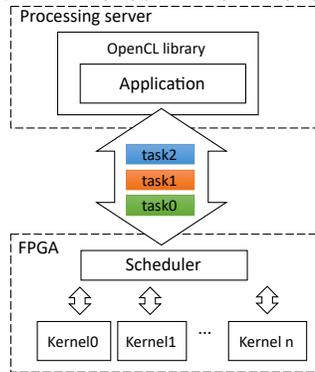
Fig. 1. System overview of the Zstd accelerator solution
