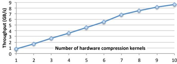
Fig. 5. Compression throughput vs number of hardware kernels
