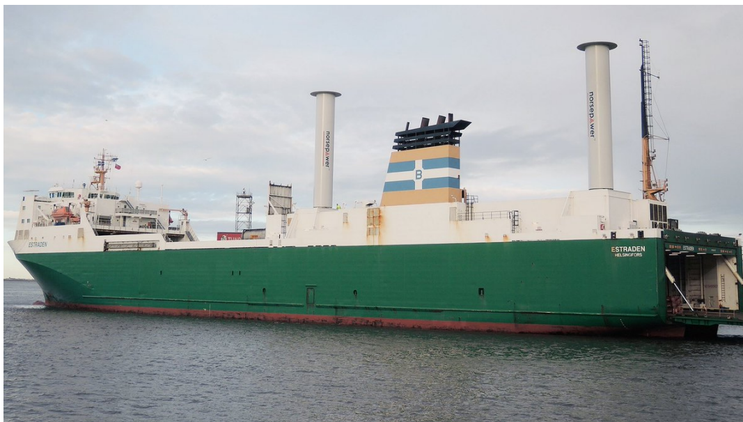
Figure 3.2: Two Norsepower Rotor Sails installed on the M/V Estraden [22].
