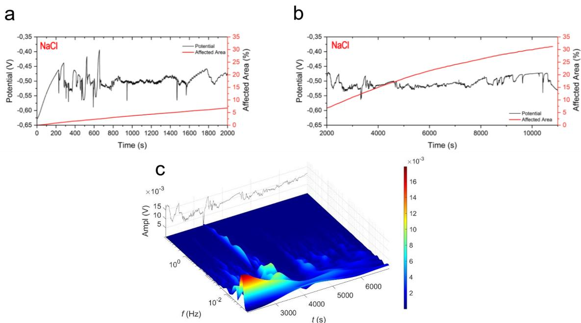
Figure 2 Raw EPN signal with change in affected area, from  $t=0-2$  ks (a) and  $2-11$  ks (b) of a AA2024 T3 micro-electrode immersed in 4.5 ml 0.05 M NaCl without inhibitor.
