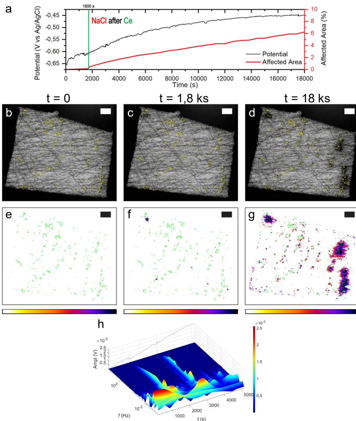
Figure 6 (a) Raw EPN data with the change in affected area of a AA2024-T3 micro-electrode immersed in 4.5 ml 0.05 M NaCl, after an initial exposure to 0.05 M NaCl with 1 mM  $\text{Ce}(\text{NO}_3)_3$ , (b-d) Microstructure (intermetallics in yellow) at  $t=0$  (b), after 1,8 ks (c) and 18 ks (d), (e-g) Activity maps (in color scale, intermetallics in green) at the same time instants, (h) CWT spectrum from  $t=0,2-5,2 \text{ ks}$
