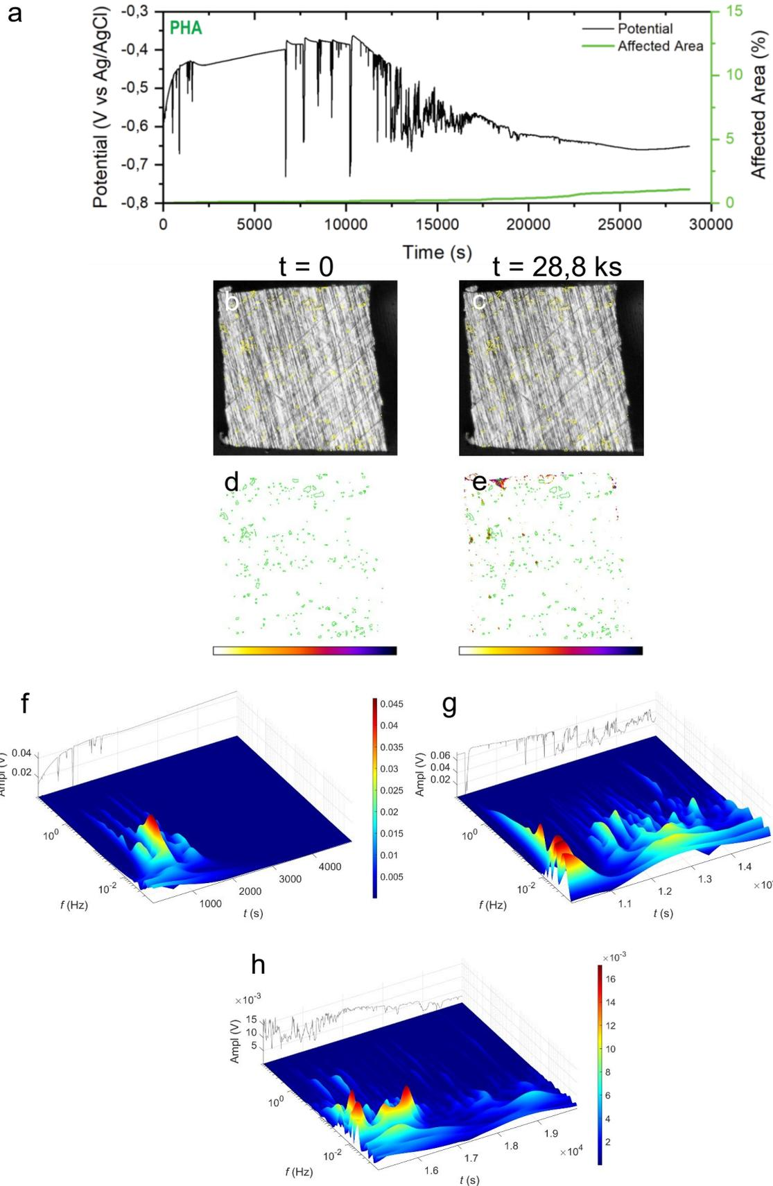
Figure 4 (a) Raw EPN signal with the change in affected area of a AA2024-T3 micro-electrode immersed in 4.5 ml 0.05 M NaCl with 1 mM PHA, (b-c) Microstructure before and after exposure (intermetallics in yellow), (d-e) Activity maps (in color scale, intermetallics in green) at the same time instants, (f-h) CWT spectra from 0-5 ks (f), 10-15 ks (g) and 15-20 ks (h)
