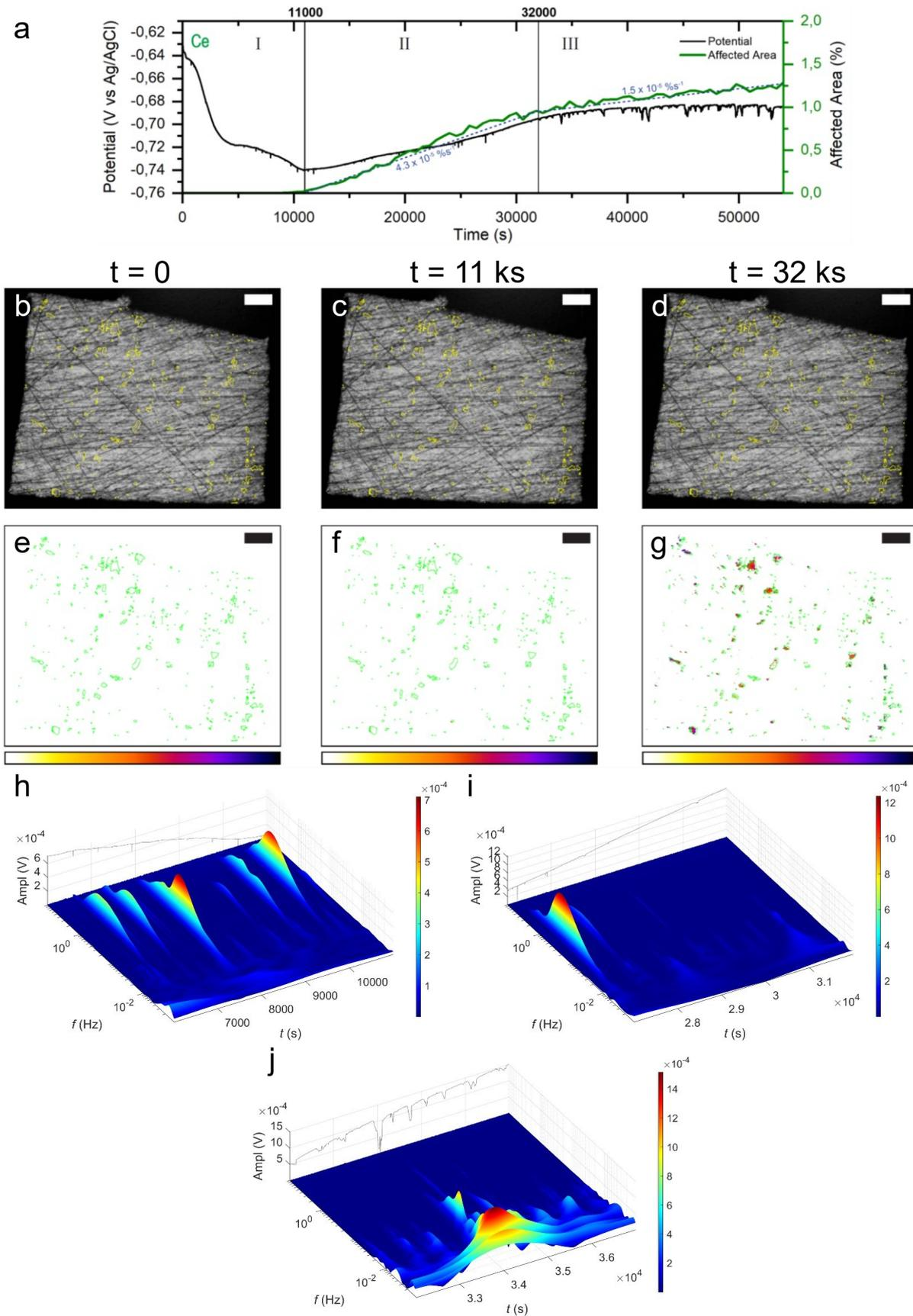
Figure 3 (a) Raw EPN data with the change in affected area of a AA2024-T3 micro-Homborg, A. M., Olgati, M., Denissen, P. J., & Garcia, S. J. (2022). An integral non-intrusive electrochemical and in-situ optical technique for the study of the effectiveness of corrosion inhibition. *Electrochimica Acta*, 403, 139619 <https://doi.org/10.1016/j.electacta.2021.139619>
