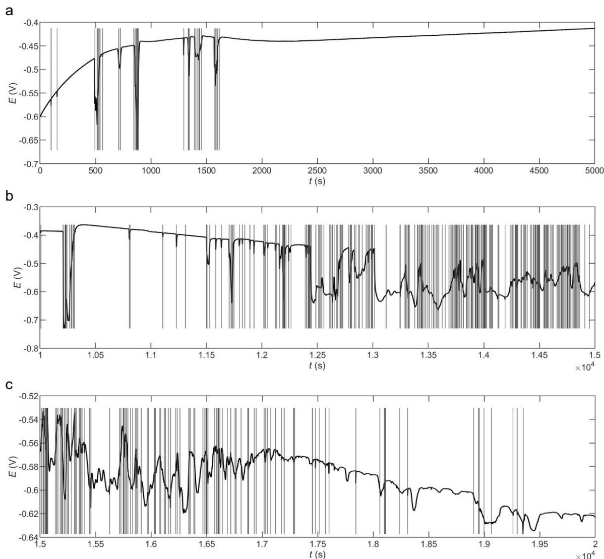
Figure 5 Raw EPN signal with transient locations indicated by grey vertical lines from 0-5 ks (a), 10-15 ks (b) and 15-20 ks (c) of a AA2024-T3 micro-electrode immersed in 4.5 ml 0.05 M NaCl with 1 mM PHA
