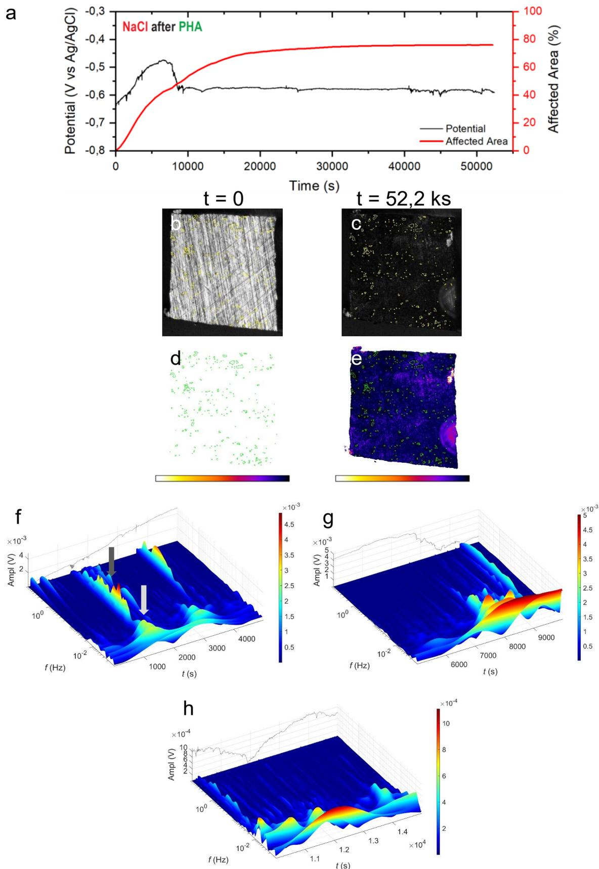
Figure 7 (a) Raw EPN data with the change in affected area of a AA2024-T3 micro-electrode immersed in 4.5 ml 0.05 M NaCl, after an initial exposure to 4.5 ml 0.05 M NaCl with 1 mM PHA, (b-c) Microstructure before and after exposure (intermetallics in yellow), (d-e) Activity maps (in color scale, intermetallics in green) at the same time instants, (f-h) CWT spectra from  $t=0-15$  ks, separated in each time 5 ks
