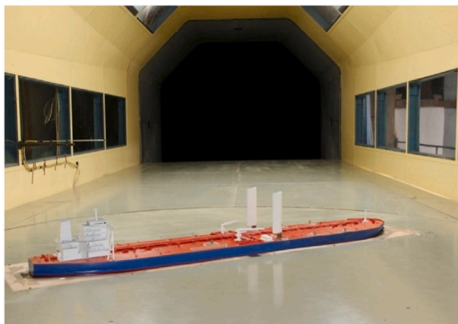
Fig. 4. The wind tunnel test for the ship adopting WAPS [51].
