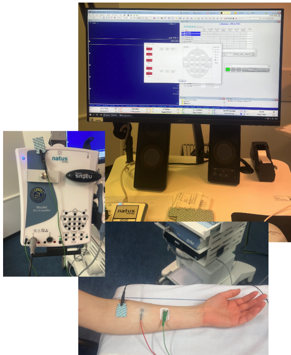
Figure 20: Impedance measurement testing set-up using the Natus Nicolet AT2+6 amplifier and the built-in impedance test. The black wire was connected to the ground electrode, the red wire to a silver cup electrode and the green wire was connected to the electrode (prototype or Ag/AgCl) of interest.
