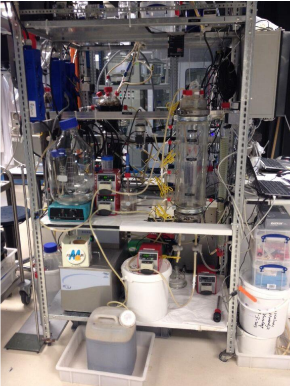
a Figure E1 Photo of the lab-scale two-phase AD system (a: Leaching bed reactor; b: UASB reactor)
