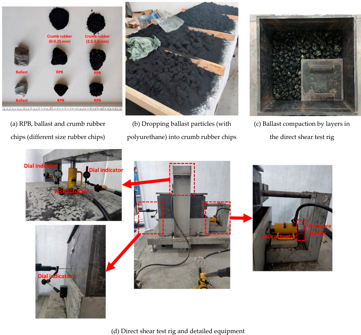
Figure 2. Direct shear tests on RPB.
