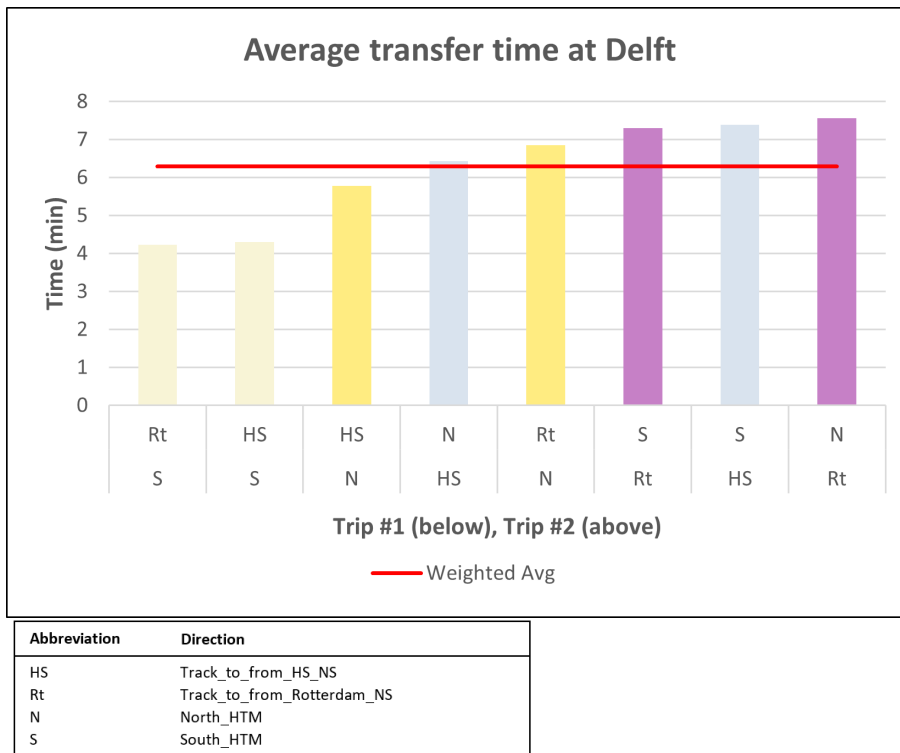
Figure 5.8: Average transfer time of the transfers at Delft between NS (train) and HTM (bus/tram) and their directions
