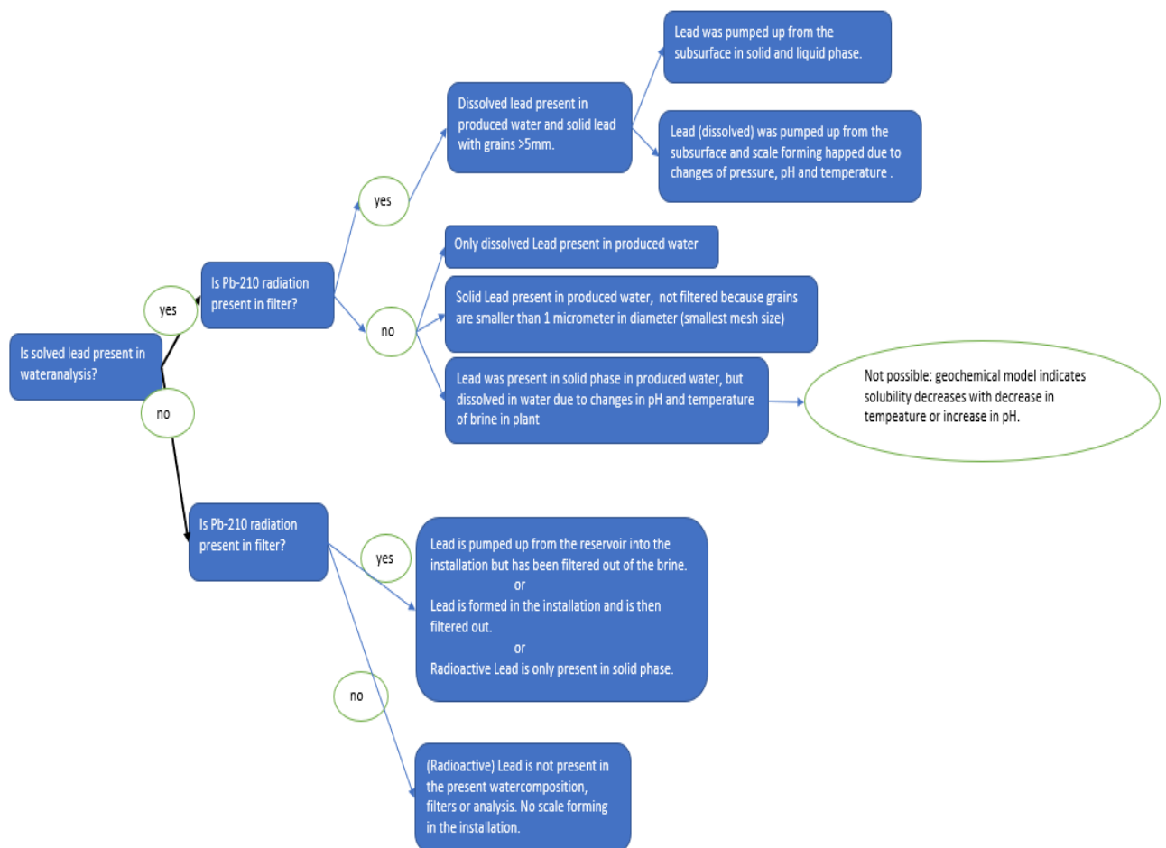
Figure 11: Flowchart of water and filter analysis regarding lead scale characterization.
