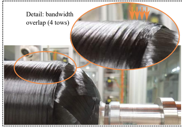
Figure 4.4: Bandwidth overlap at the turnaround location of circumferential plies.
