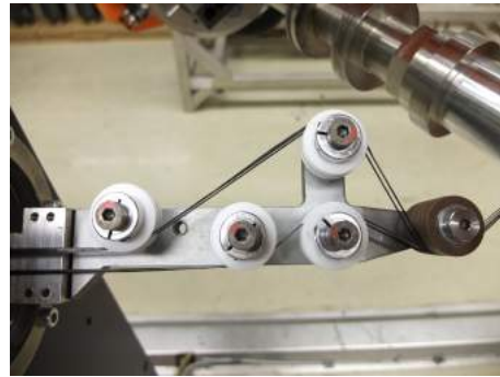
Figure 2.5: Overview of rollers installed on the filament winding eyelet.
