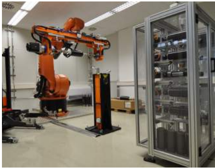
Figure 2.4: KUKA KR-500 robot for filament winding at cellcentric GmbH.
