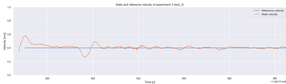
Figure 4.9: Reference and state velocity of the Tito Neri Dark Blue for the Port Call experiment (Strategy: Time, Berth available: Yes, Alternative: 7)
