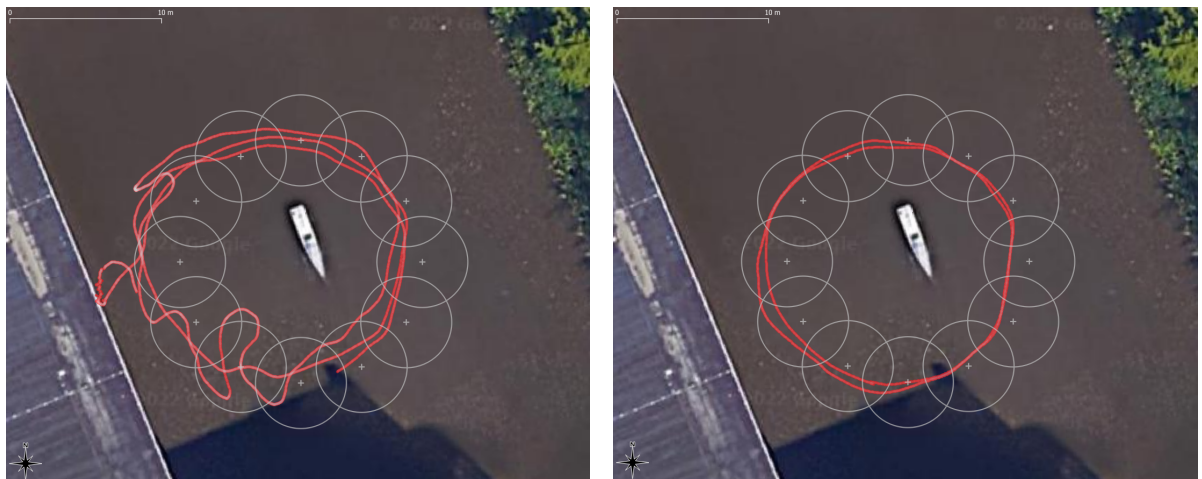
Figure 4.1: Sailed paths of the Tito Neri Dark Blue during Experiment Green Routing (left: 800 RPM, right: 1200 RPM). The grey circles represent the waypoint acceptance criteria. If the vessel moves within this radius, it is considered to have reached the waypoint and the next one is generated
