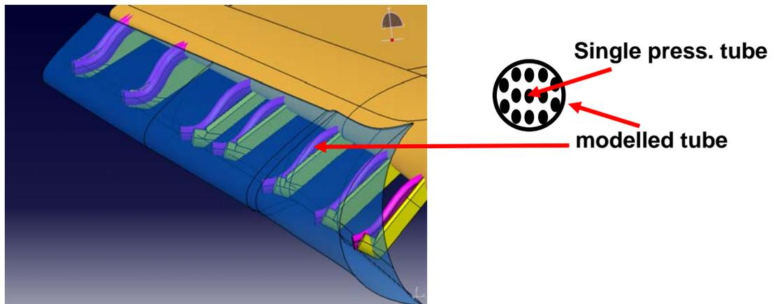
Figure 1: Pressure tube bundles on the EUROLIFT II high-lift configuration
