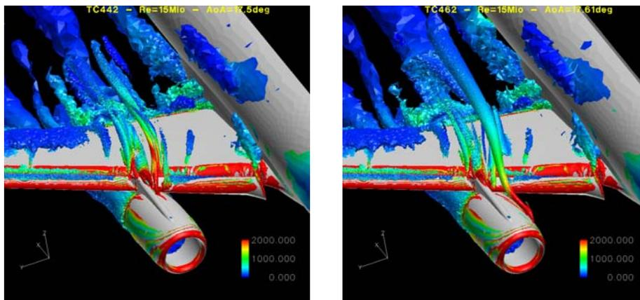
Figure 3: Structure of the generated vortices for stage II (left) and stage III (right) at ETW-conditions
