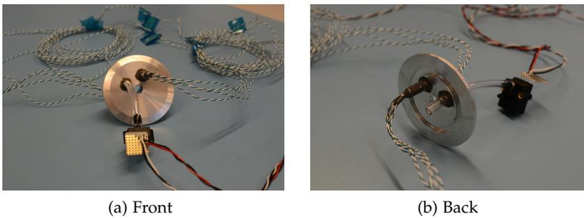
Figure 41: Photos of the vacuum transition flange.
