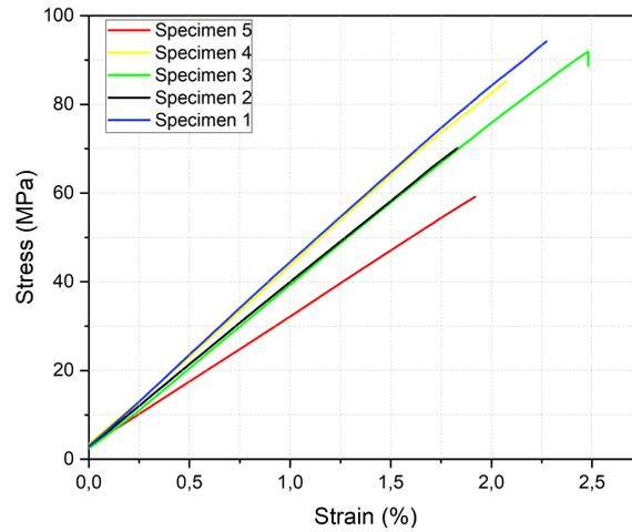
(b) Stress-Strain Curve of Flexural Testing of PHTE system
