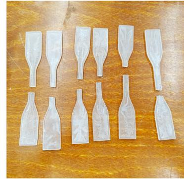
(c) Failed Specimen for flexural testing of Epikote system
