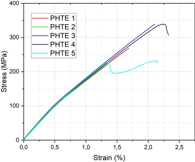
(b) PHTE/Epikure04908-based composite stress-strain
