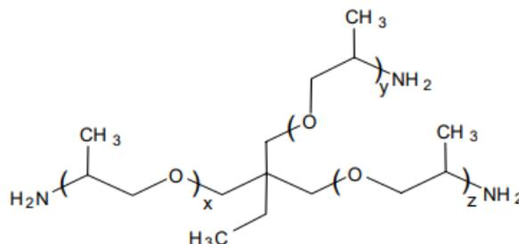
Figure 4.5: Chemical Structure of Jeffamine T403 Polytheramine
