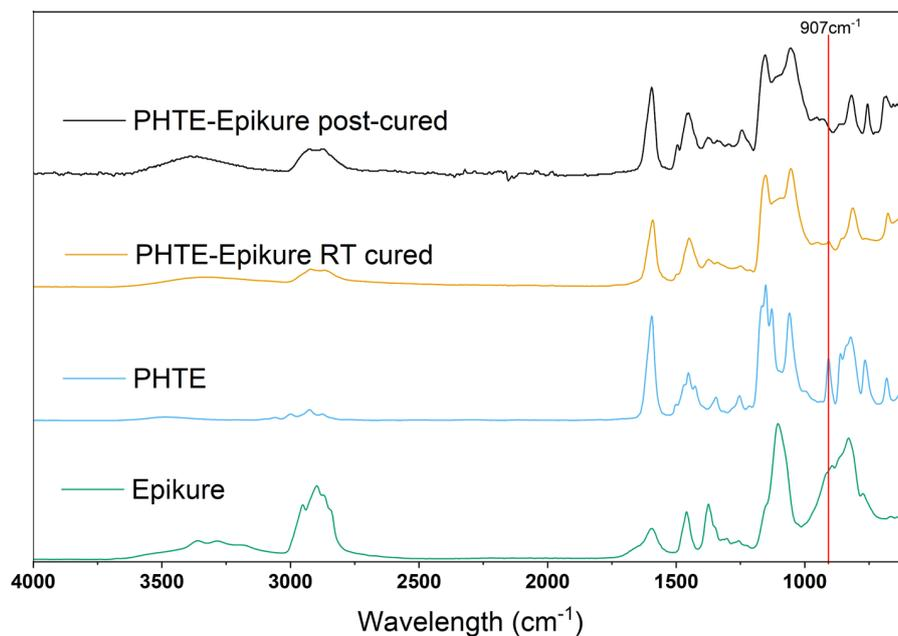
Figure 5.10: FT-IR spectra of PHTE, Epikure, and PHTE/Epikure04908 cured resin systems
