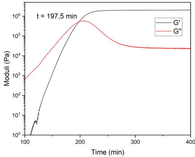
Figure 5.13: Storage ( $G'$ ) and Loss ( $G''$ ) modulus over time
