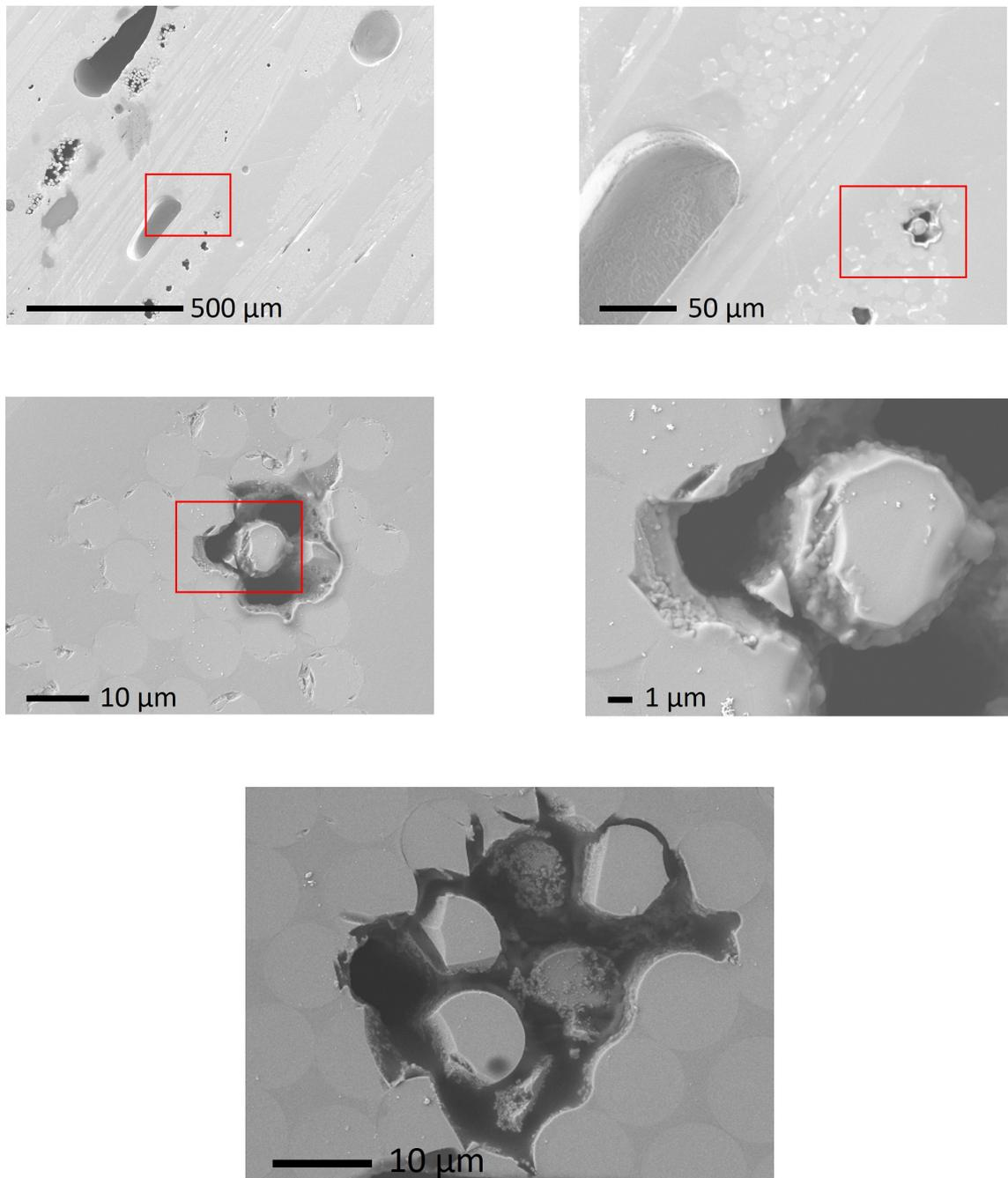
Figure 5.22: Scanning Electron Microscopy of the PHTE/Epikure04908 based laminate
