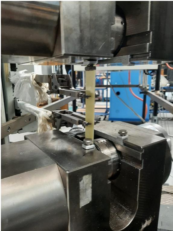
(a) PHTE/Epikure04908 tensile test configuration
