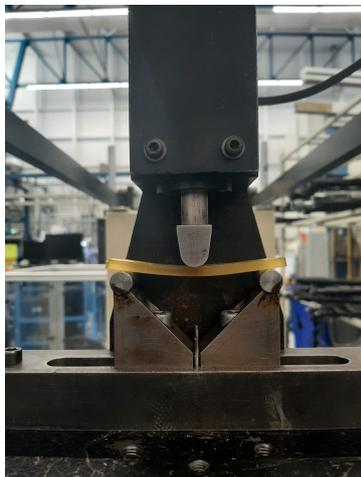
(a) Flexural testing of resin
