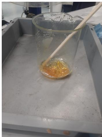
**Figure 4.16:** Cured PHTE/Epikure04908 system as a result of the silicon heat bath
