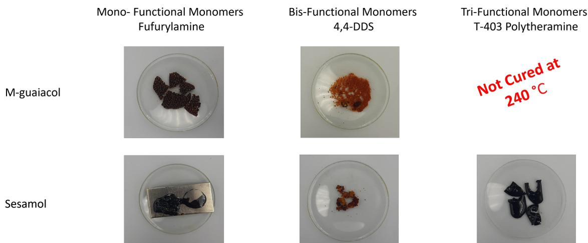
**Figure 5.3:** Cured Benzoxazines at 220 °C for 4 hours
