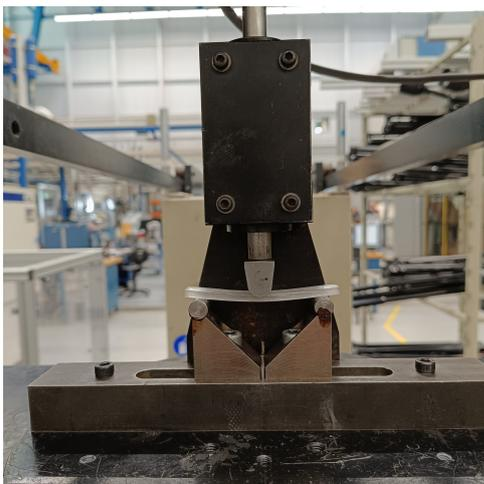
(a) Flexural testing of Epikote system
