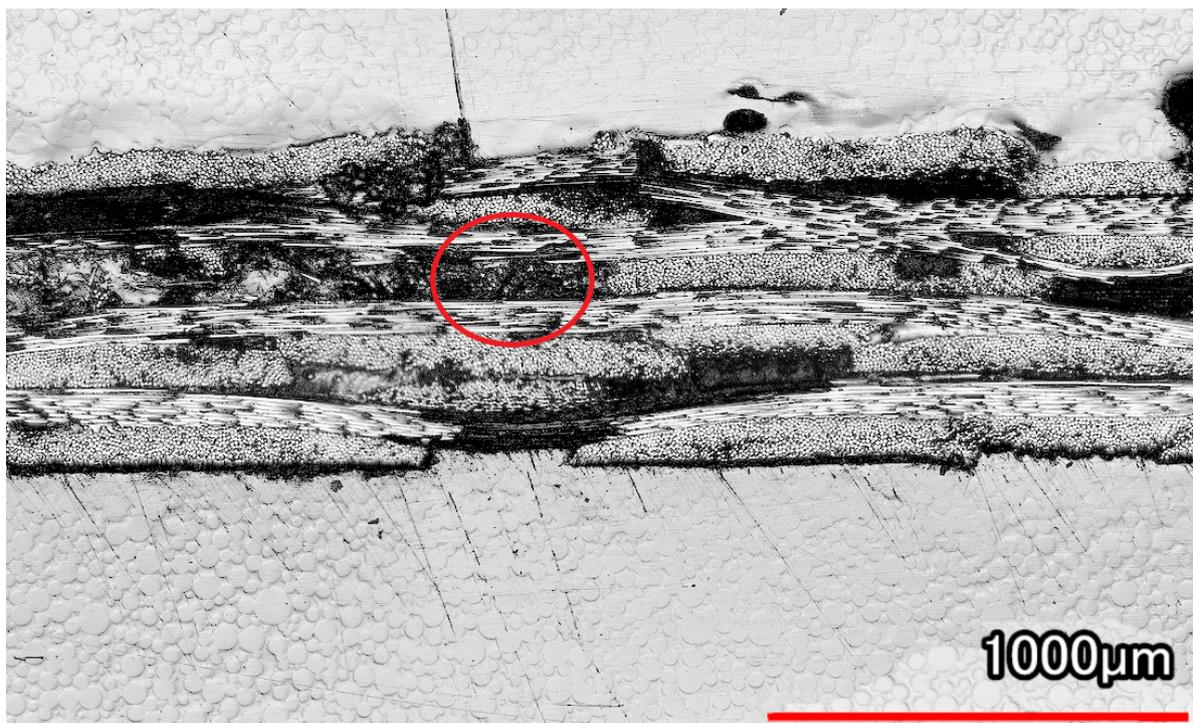
Figure 5.6: Laser Microscopy image of BS3-based laminate
