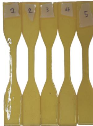
Figure 4.13: PHTE/Epikure04908 tensile specimen
