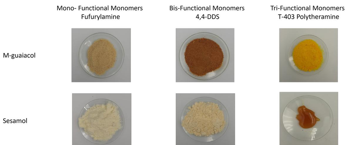
**Figure 5.1:** Synthesized bio-based Benzoxazine monomers
