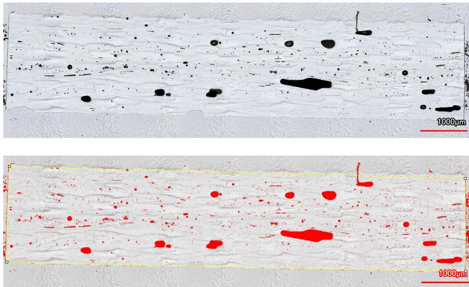
**Figure 5.21:** Laser microscopy images of the composite and analyzed images through ImageJ software by altering the threshold to obtain void content.
