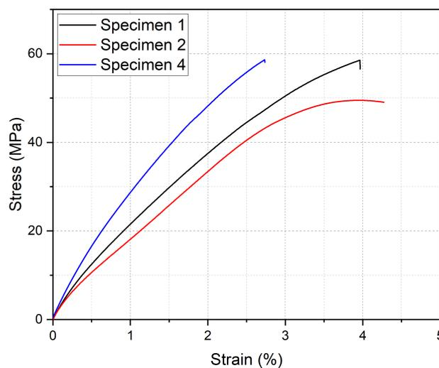
(a) Stress-Strain Curve of Tensile Testing of PHTE system
