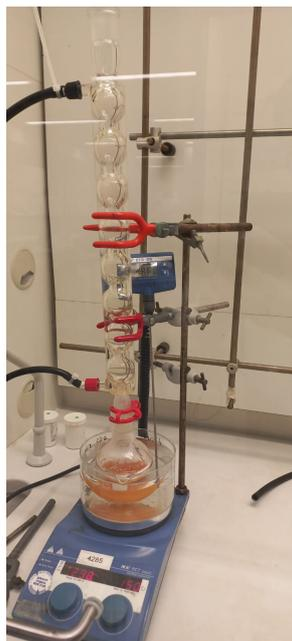
**Figure 4.7:** Synthesis of initial benzoxazine monomer in reflux
