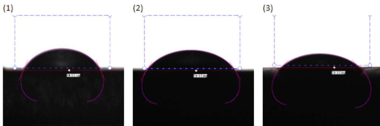
Figure 5.8: Water Contact Angle on PHTE/Epikure04908 resin specimen
