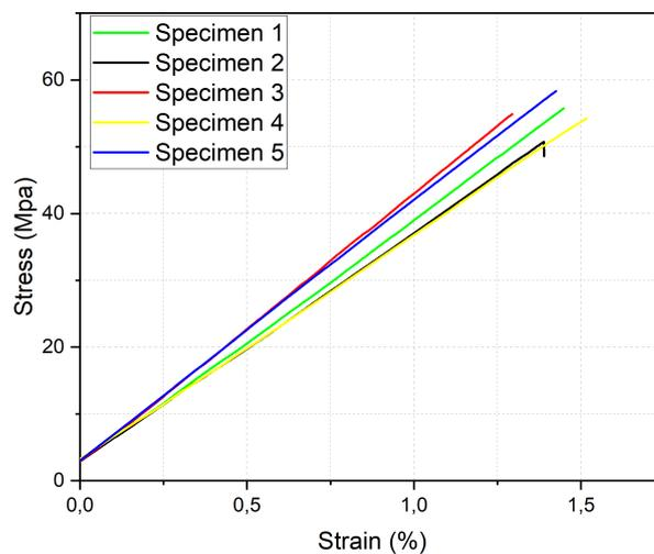
(b) Stress-Strain Curve of Flexural Testing of Epikote system
