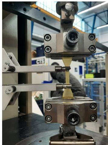
(b) Tensile testing of resin
