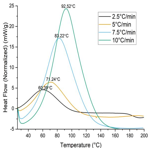
(a) DSC runs for PHTE-Epikure04908 mix in 2:1 ratio at different heating rates
