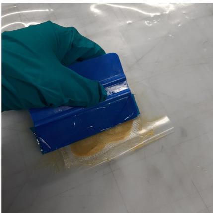
(a) Applying the resin in a single application
