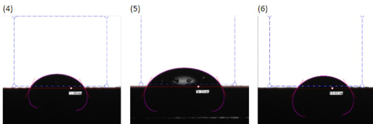
Figure 5.9: Water Contact Angle on PHTE/Epikure04908 composite specimen
