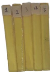
**Figure 4.13:** PHTE/Epikure04908 flexural specimen
