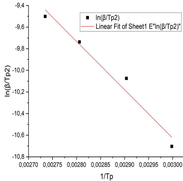
(b) Linear fit using Kissinger model to determine the activation energy of the curing reaction
