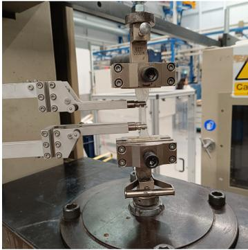
(a) Tensile test set-up of Epikote/Epikure system
