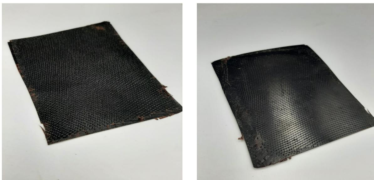
(a) Small laminate  $[0, 90, 0, 90]_s$  based on B3
