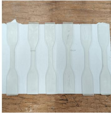
(b) Specimen for tensile testing of Epikote system
