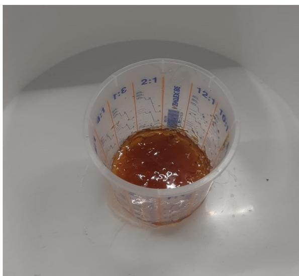
Figure 4.10: PHTE-Epikure04908 mixture in Degassing Chamber
