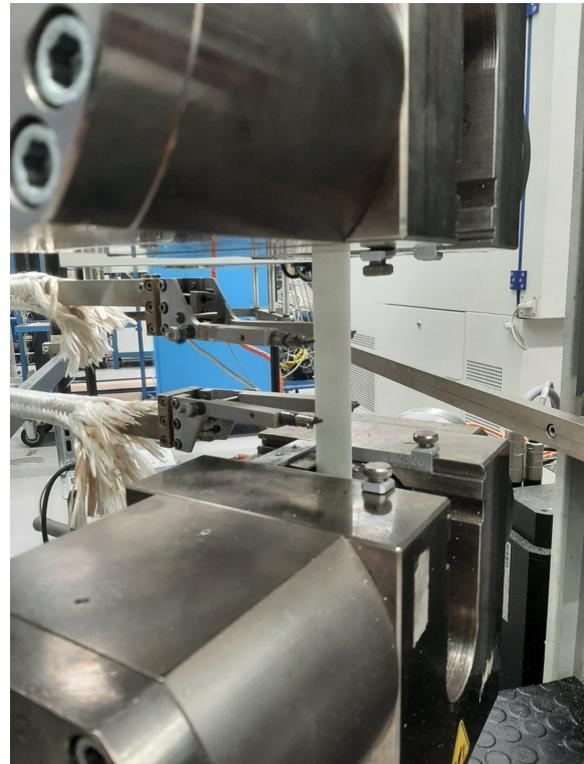
(b) Epikote/Epikure04908 tensile test configuration
