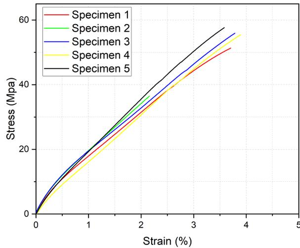
(a) Stress-Strain Curve of Tensile Testing of Epikote system
