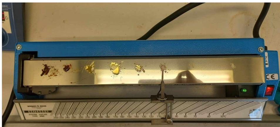
**Figure 5.2:** Koffler test used for determining optically the curing behavior of benzoxazines
