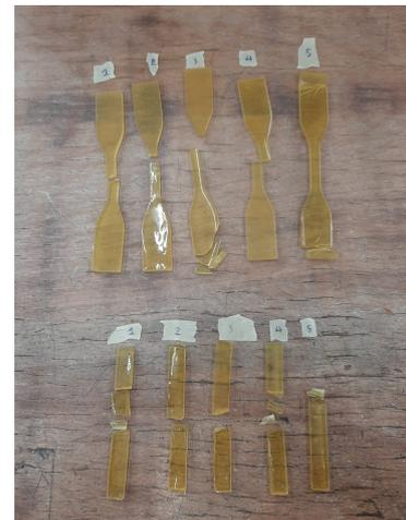
(c) Specimens after failure
