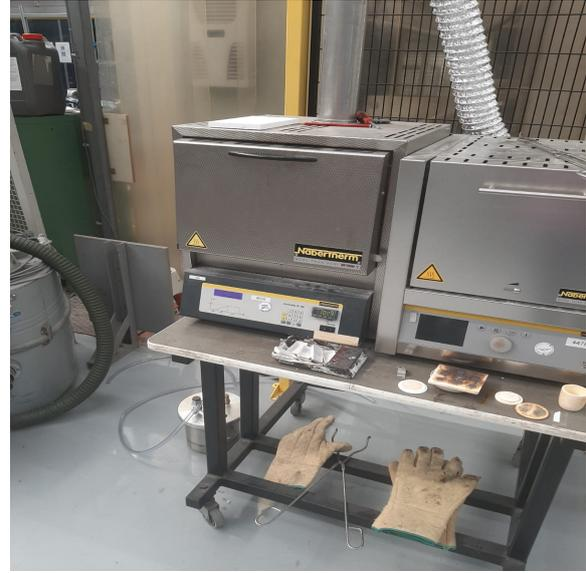
(b) Vacuum furnace used for burning of the resin
