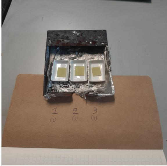
(a) PHTE composite samples used for burn-Off test
