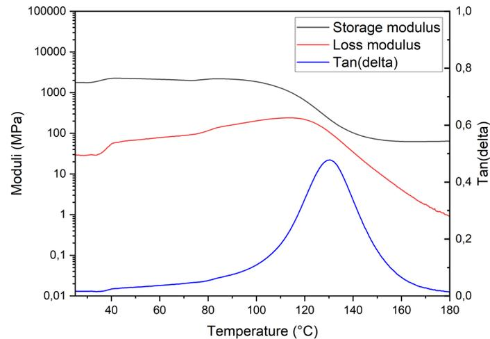
(a) PHTE-Epikure04908 system post cured at 140 °C for 1 hour
