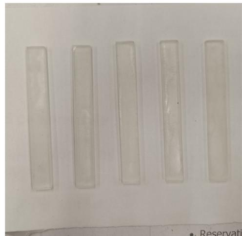
(b) Specimen for flexural testing of Epikote system
