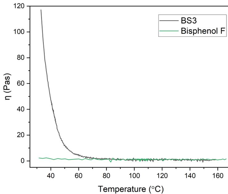
Figure 5.5: Viscosity of BS3 over temperature
