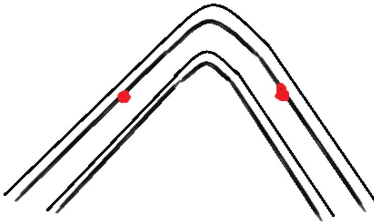
Figure 17: Picking points at the same side of the geological layer, at opposite sides of the fold.
