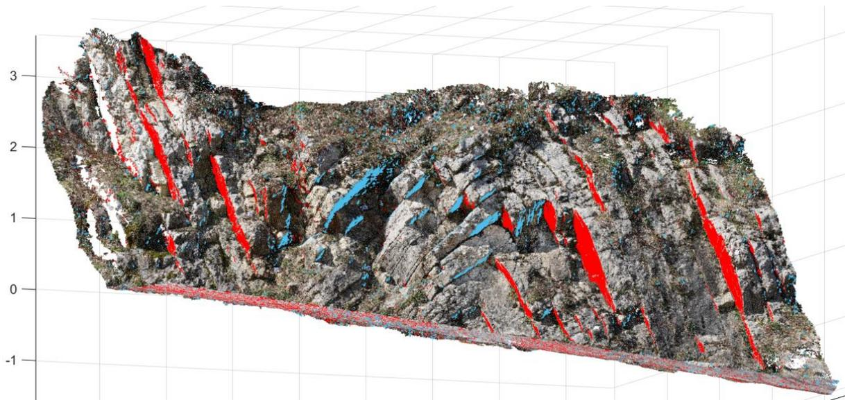
*Figure 37: fold limbs identification. Light blue colors indicate the identified first side of the fold bedding layers and the red colors indicate the other orientation of the bedding layers at the other side of the fold.*
