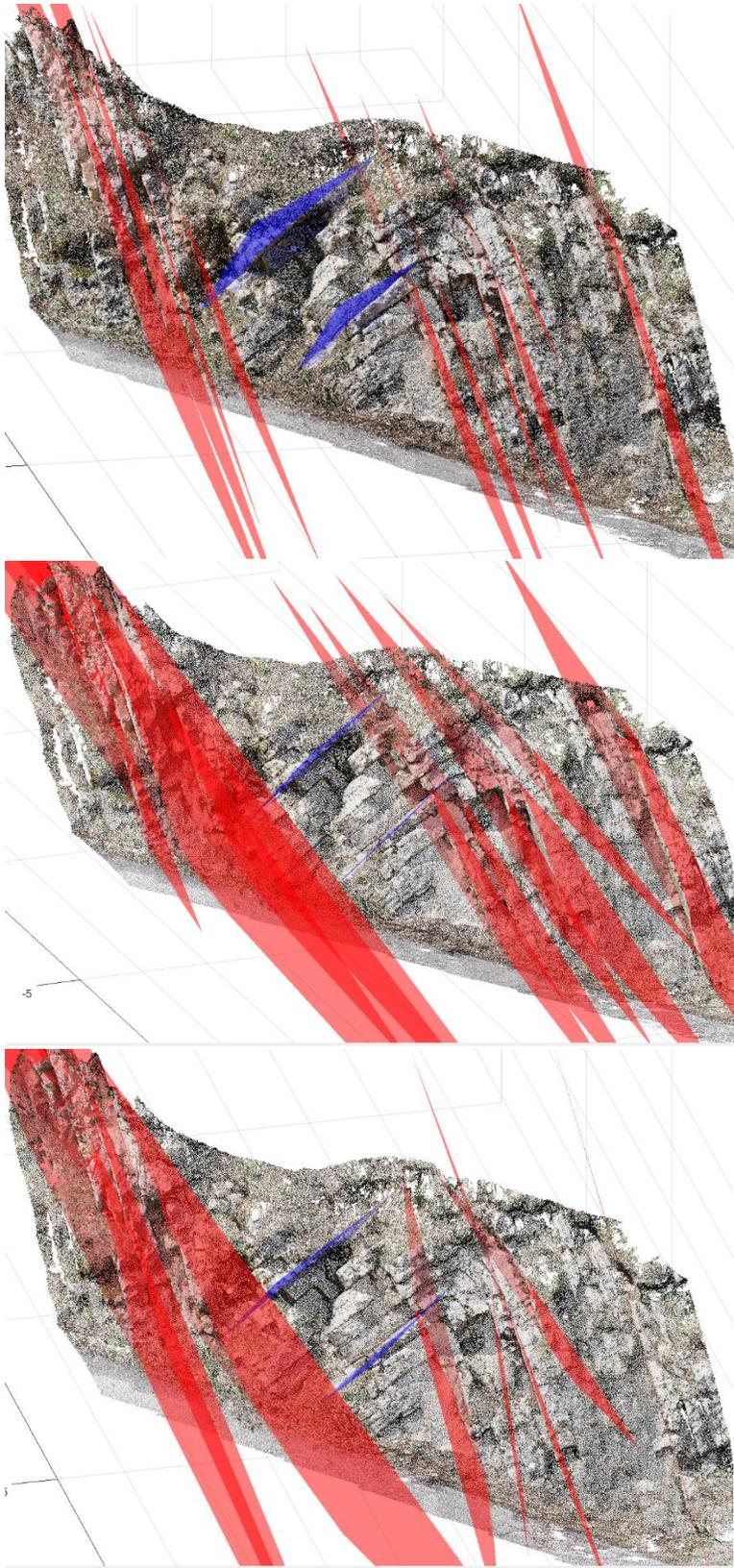
Figure 7: Angular difference plane fitting. 1 degree, 5 degrees and 10 degrees.
