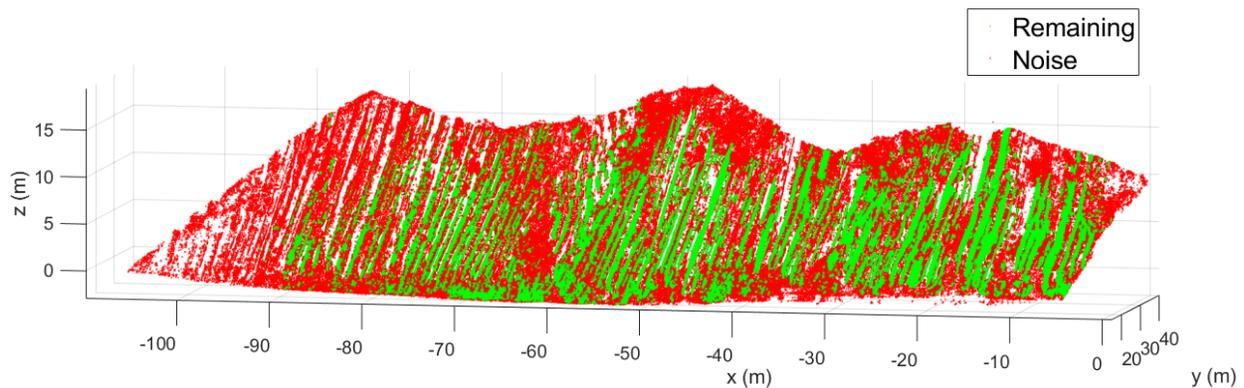
Figure 28: Noise removal global image. Red are points which are removed because they are classified as noise. Green points are kept since they are not classified as noise.
