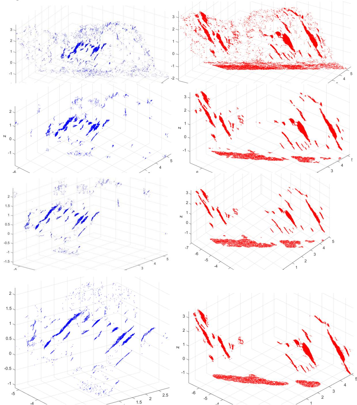
Figure 47: Horizontal downwards are shown the original pointcloud selection (with directional filter and roughness filter), the 50 neighbors result, the 100 neighbors result and the 500 neighbors result
