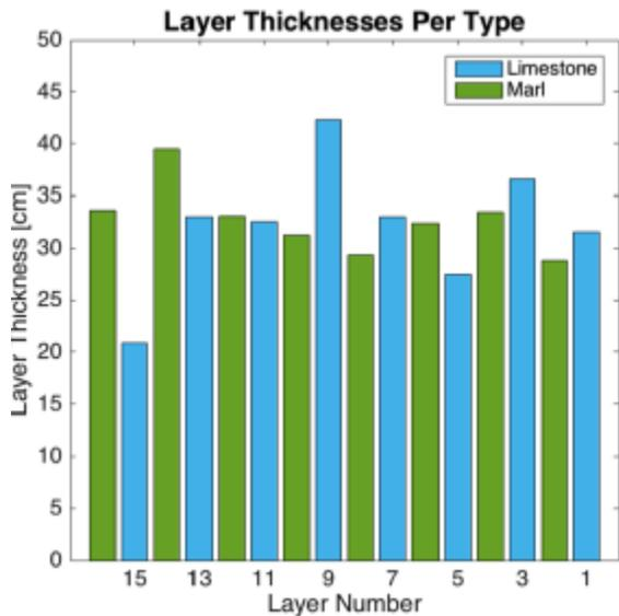
Figure 41: layer thickness for Limestone and Marl layers.
