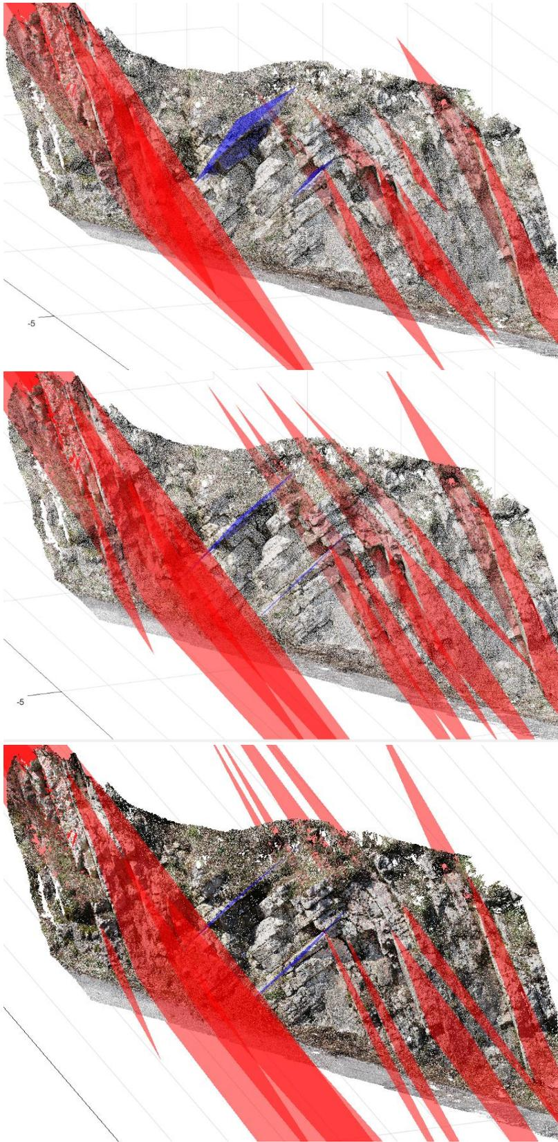
Figure 6: Maximum distance plane fitting. 7 cm, 15 cm and 25 cm.
