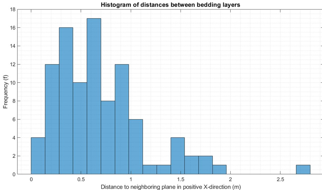
Figure 44: Histogram of computed layer thickness.
