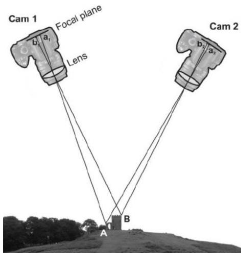
Figure 8: photogrammetry principle, found in Walstra (2007)
