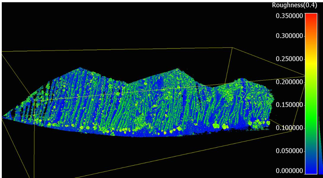
Figure 22: Roughness calculation with a kernel size of 0.4 meters.
