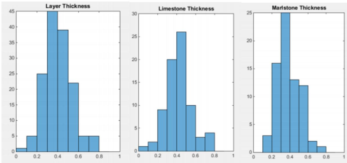
Figure 40: histogram of layer thickness (in meters).
