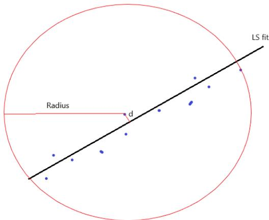
Figure 11: Sketch of roughness calculation.
