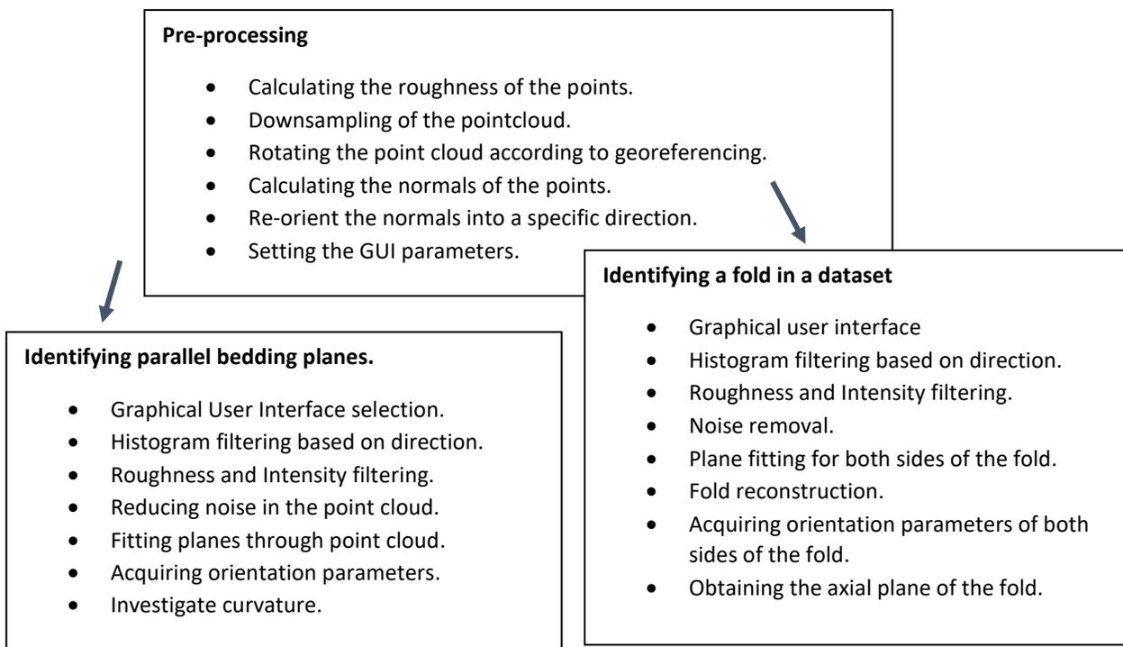
Pre-processing is a step which happens no matter the dataset. Then depending on if only parallel bedding planes are to be identified or a fold needs to be identified, different sets of processing steps are performed.
