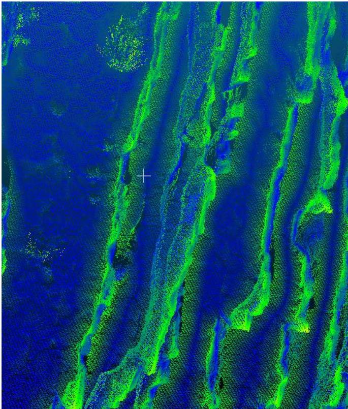
*Figure 15: Green values represent high roughness points and blue values represent low roughness points. The points are located at resp. the face on of the layers and the bedding of the layers.*
