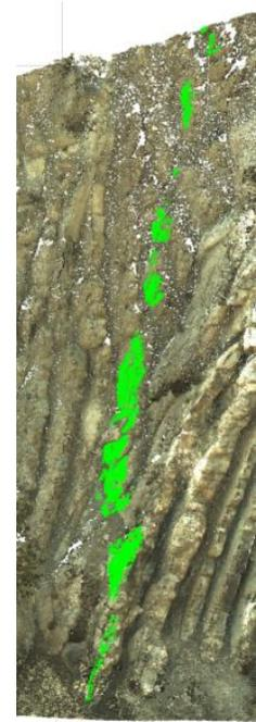
Figure 36: Example of commission errors in plane fitting algorithm.
