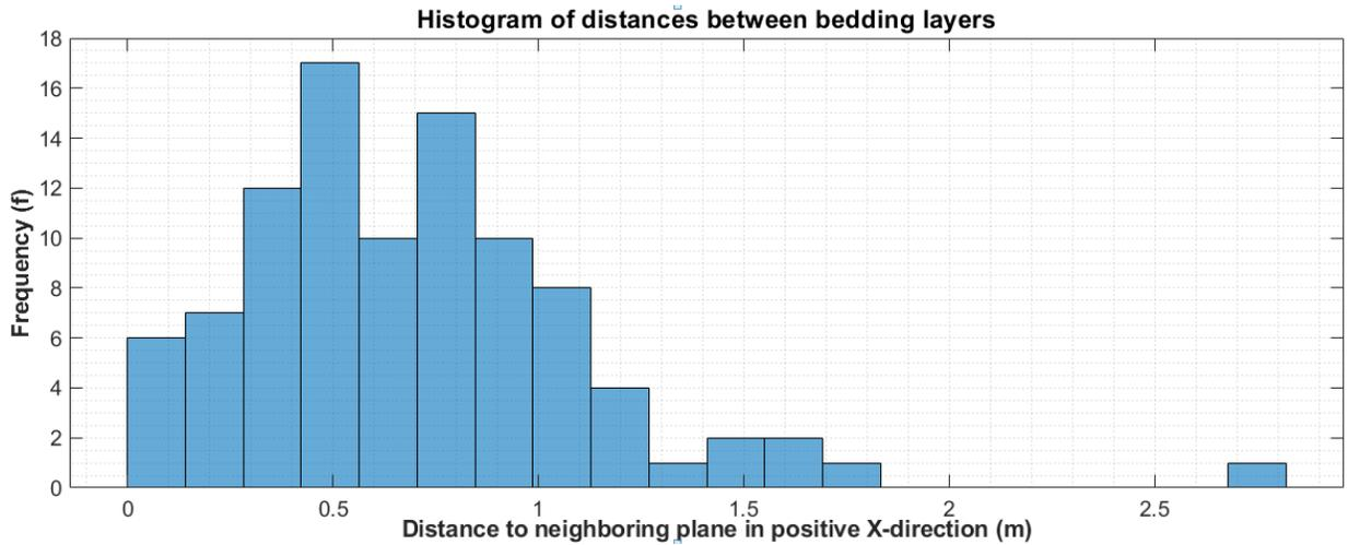
Figure 33: Histogram of distances between the fitted planes
