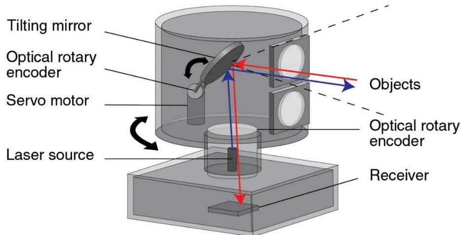
Figure 9: LiDAR principle [5]
