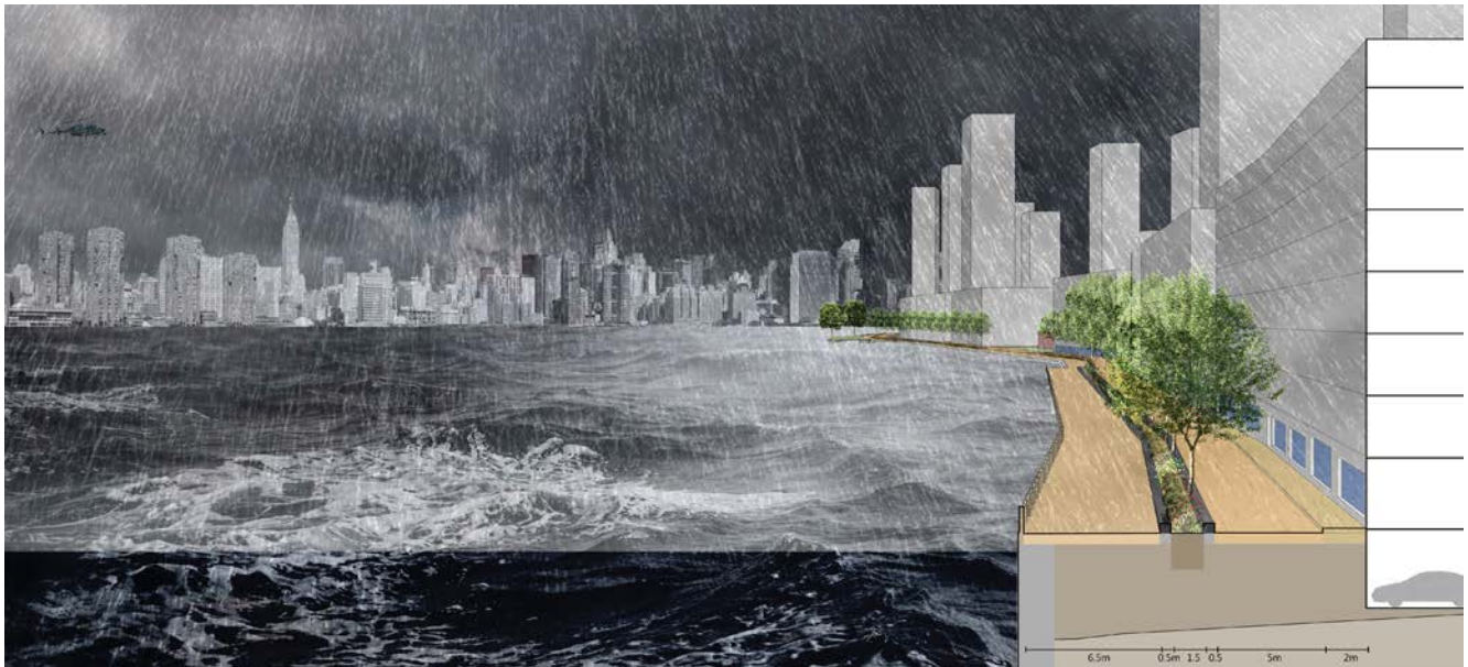
27 The raised bulkhead protecting the buildings from a 1/500 storm surge in 2050
