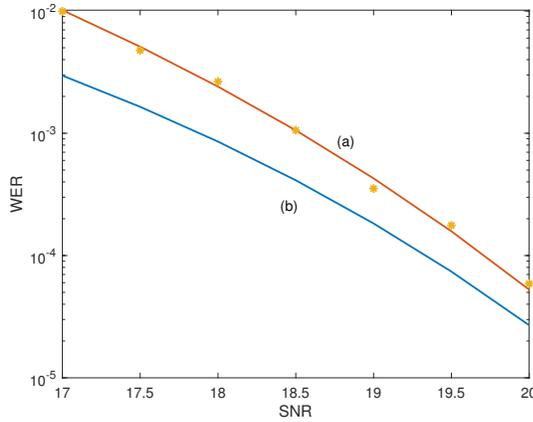
Fig. 3. Word error rate, WER versus SNR =  $-20 \log(\sigma)$  (dB) of the new detection method computed using (a) union bound (23), (b) union bound estimate (25), and by simulations. The points marked with ‘\*’ result from simulations. Note that Curve (a) is the same as Curve (b) in Figure 1. For all curves,  $n = 12$ .
