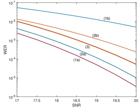
Fig. 4. Word error rate, WER versus SNR =  $-20 \log(\sigma)$  (dB) of (1a) Euclidean detection, no offset; (1b) Euclidean detection,  $b_0 = 0, b_1 = 0.025$ ; (2a) Pearson detection, no offset; (2b) Pearson detection,  $b_0 = 0, b_1 = 0.025$ ; (3) new detection method, with and without offset. For all curves,  $n = 12$ .
