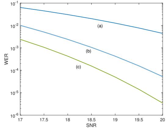
Fig. 1. Word error rate, WER versus signal-to-noise ratio,  $\text{SNR} = -20 \log(\sigma)$  (dB). Curve (a) shows Euclidean detection with channel mismatch,  $b_0 = 0.1$ ,  $b_1 = 0.01$ , Curve (b) shows the new detection method, which is detailed in Section III, and Curve (c) shows Euclidean detection for the ideal AWGN channel, no mismatch,  $b_0 = b_1 = 0$ . All curves for  $n = 12$ .
