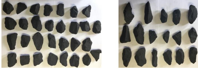
Figure 4 Flaky (left) and elongated (right) ballast particles in particle size range of 25~35 mm
