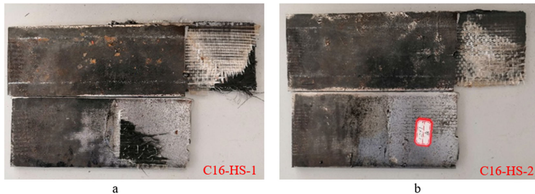
Figure 5. Failure modes of single-side reinforcement: a) FRP rupture; b) interfacial debonding and cohesion failure.
