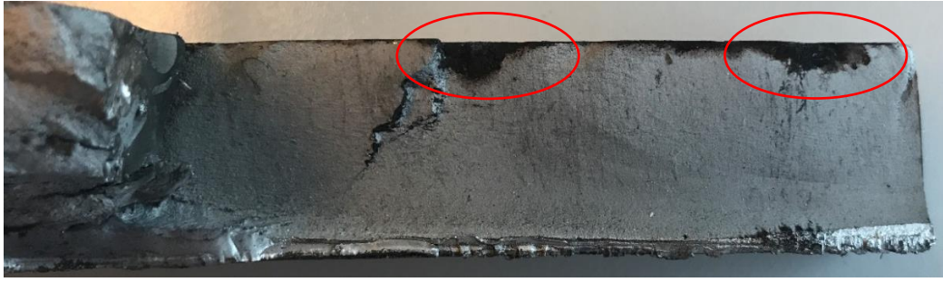
Figure 13 Highly corroded areas at the crack initiation locations on the fracture surface of base material failure in S890.
