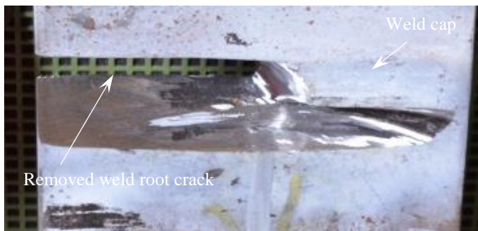
Figure 7. Removal of the crack at the weld toe of the weld root.
