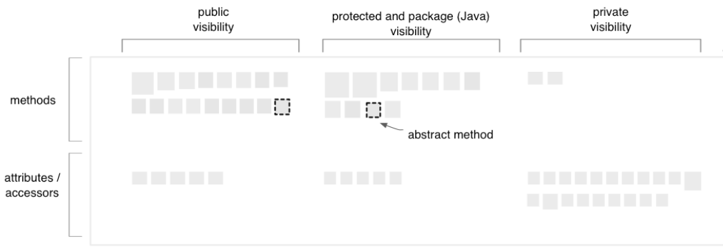
Figure 3.5: Polymetric class view from inFusion. Image taken from help files.
