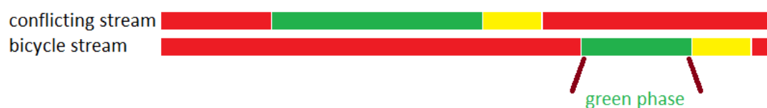
Figure 3-5: Consequence of extension or no extension of conflicting streams for green times of cyclists
