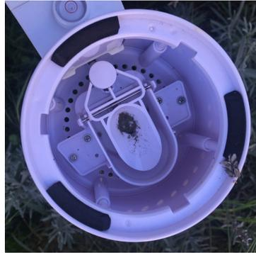
**Figure 11:** Bucket partly filled with sand and organic material.
