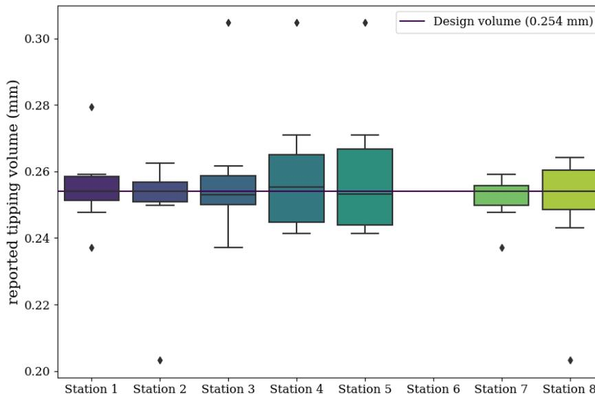
**Figure 16:** Results of tipping volume experiment A. The result is shown for seven different stations, leaving station 6 untested. The box plots are based on 9-10 values per stations. The horizontal line represents the designed bucket volume of 0.254 mm, or 0.01 inch.
