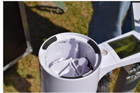
(b) Testing of tipping bucket mechanism
