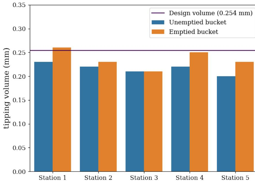
**Figure 17:** Results of tipping volume experiment. The result is shown for 5 different stations, tested with unemptied and emptied buckets. The bar graphs show the mode of the experiment, that was carried out 5 times for each station.
