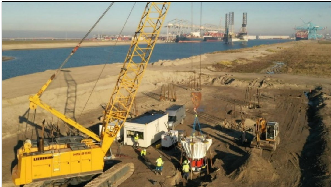
Figure 1: Lifting the load test frame into place at the Amaliahaven test site
