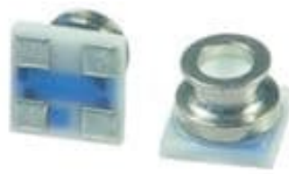
Figure 3.8: MS5837-30BA sensor without the wires showing the metal round case
