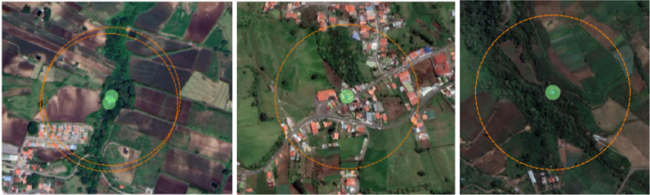
Figure 24: Springs Rodillal, Edwin Coto and Oscar Are. The orange circle represents the by-law-determined protection zone with a 200-m radius. Urban and agricultural activity are clearly located within the protection zone.
