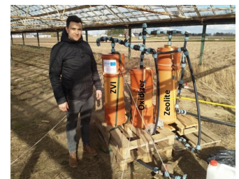
Figure 11: A zero-valent filter system
