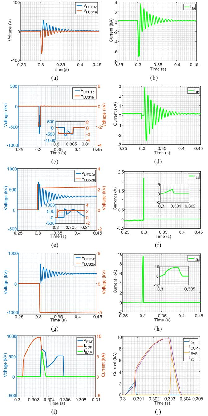
Fig. 12. Current and Voltage at the paths of MLB1: (a) Voltages on “healthy” NCP 1a; (b) current on “healthy” NCP 1a; (c) voltages on “healthy” NCP 1b; (d) current on “healthy” NCP 1b; (e) voltages on “faulty” NCP 2a; (f) current on “faulty” NCP 2a; (g) voltages on “faulty” NCP 2b; (h) current on “faulty” NCP 2b; (i) CCP and EAP path; (j) Total breaker fault current.
