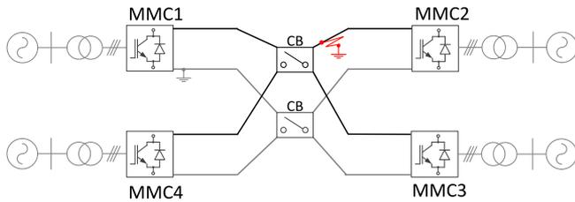
Fig. 8. Layout of the analyzed radial MTdc network with 4 terminals with a pole-to-ground dc fault.
