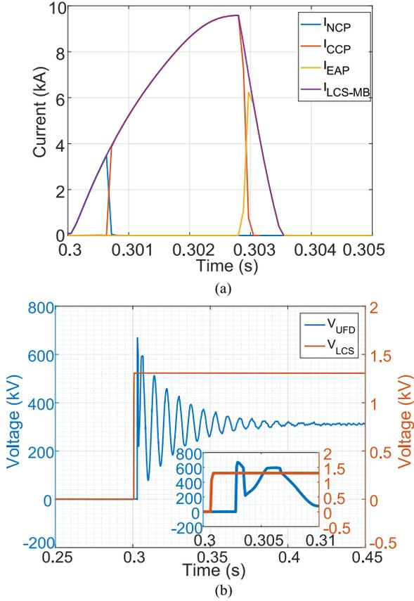
Fig. 11. LCS-MB: (a) current on the breaker paths; (b) voltage stresses on the NCP switches.
