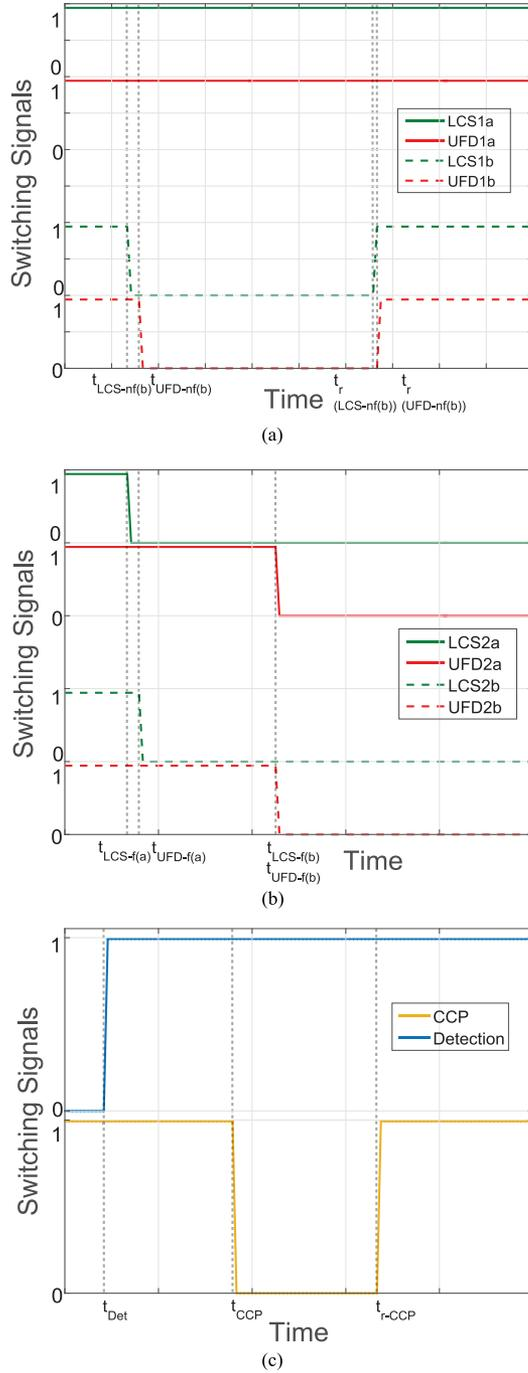
Fig. 6. Pole-to-ground - Switching Sequence MLB1: (a) Healthy line path (1); (b) Faulty line path (2); (c) Main Breaker path and Fault signals. “1” and “0” values indicate the “on” and “of” states respectively.
