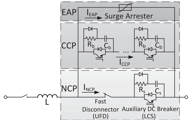
Fig. 3. LCS-MB breaker with its three paths.
