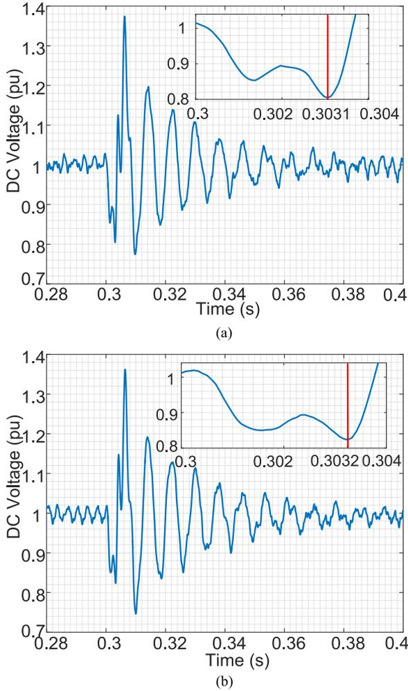
Fig. 13. DC voltage at MMC1: (a) LCS-MB; (b) MLB. The red line indicates the time at which the dc voltage starts to recover in each case.
