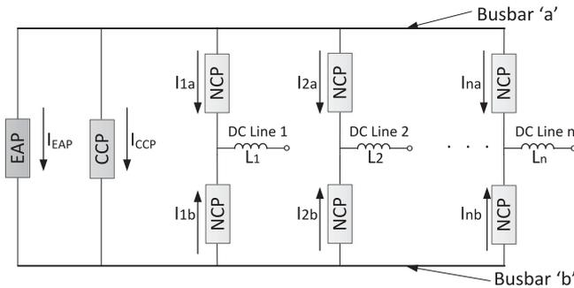
Fig. 2. Hardware structure of a Multi-line breaker (MLB).
