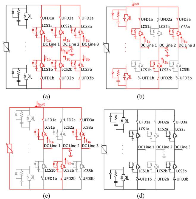
Fig. 5. Control sequence of the MLB illustrated for a configuration with three attached lines.
