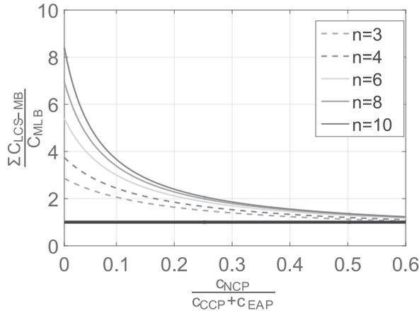
Fig. 7. Sensitivity analysis of the cost of MLB over LCS-MB breakers and cost ratio between NCP and the combined cost of CCP+EAP, for different number of lines  $n$ . The thick black line, at  $y=1$ , indicates the break-even point between the two breaker costs.
