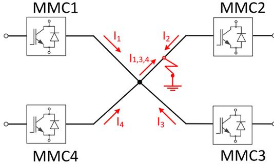
Fig. 10. Current direction during a dc fault [34].
