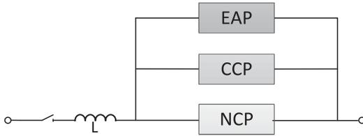
Fig. 1. Hardware structure of a hybrid breaker.
